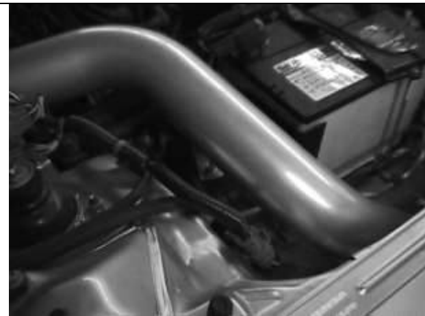
Fig 11: Intake pipe installed. Note mounting bolt.
