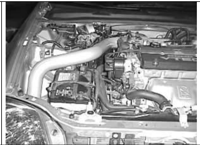
Fig 8: Intake tube installed
