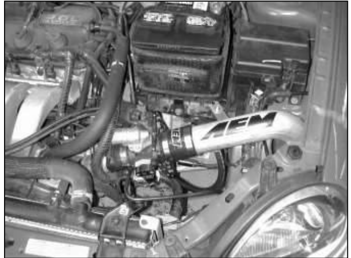
AEM® intake system installed
