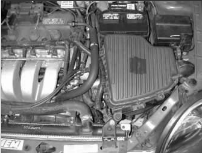
Factory airbox system installed
