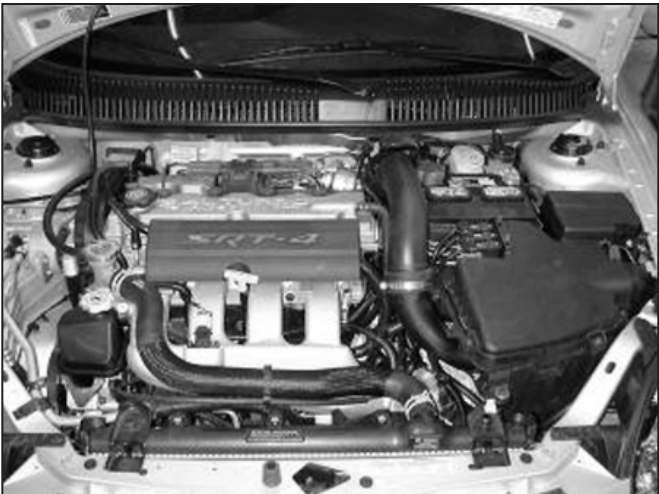
c. Remove the inlet air tube to the turbo.
