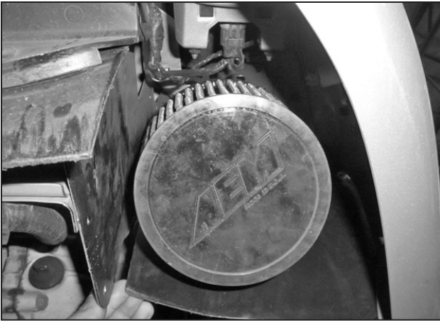
v. Attach the AEM air filter element and secure to the lower intake tube.
