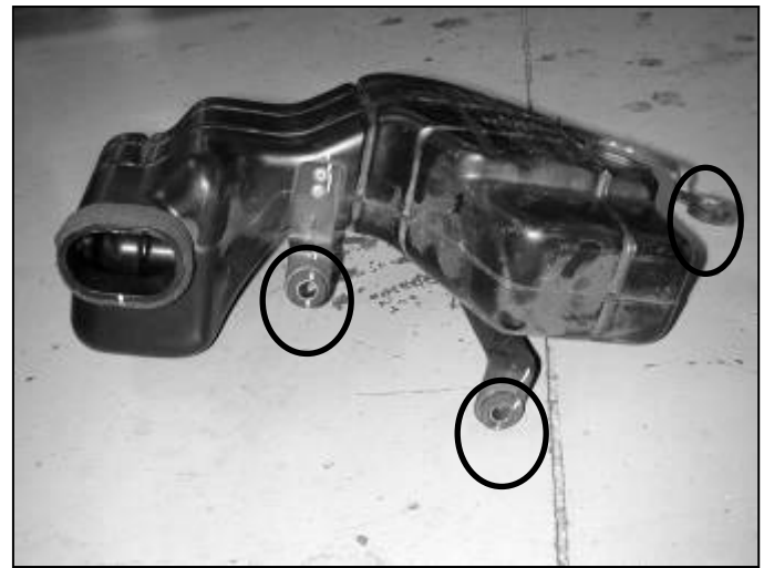
h. Loosen the three bolts that secure the lower air box and remove from the vehicle.
