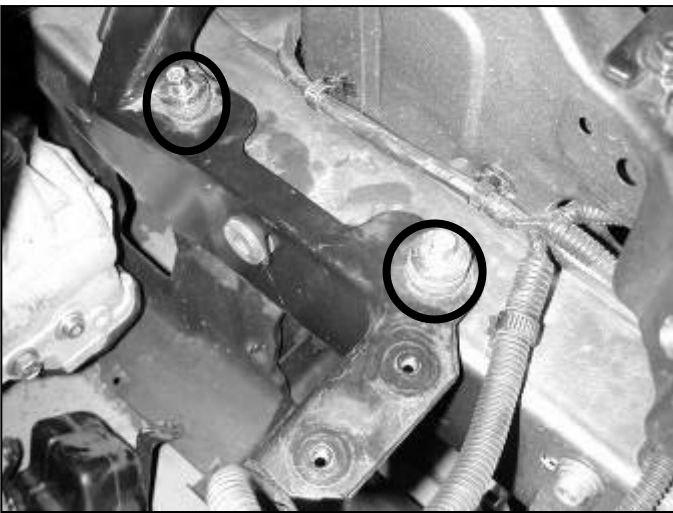
g. Remove lower mounting bracket.
