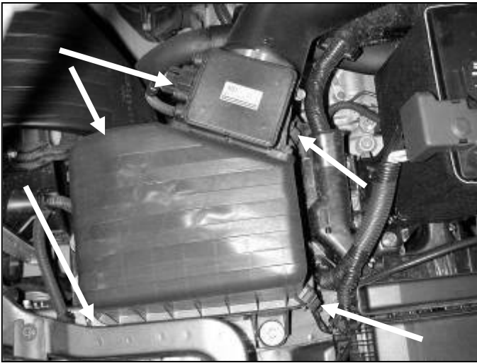
c. Unplug the MAF sensor. Remove the stock inlet pipe. Release four clamps on the air box and remove the upper air box from the vehicle.
