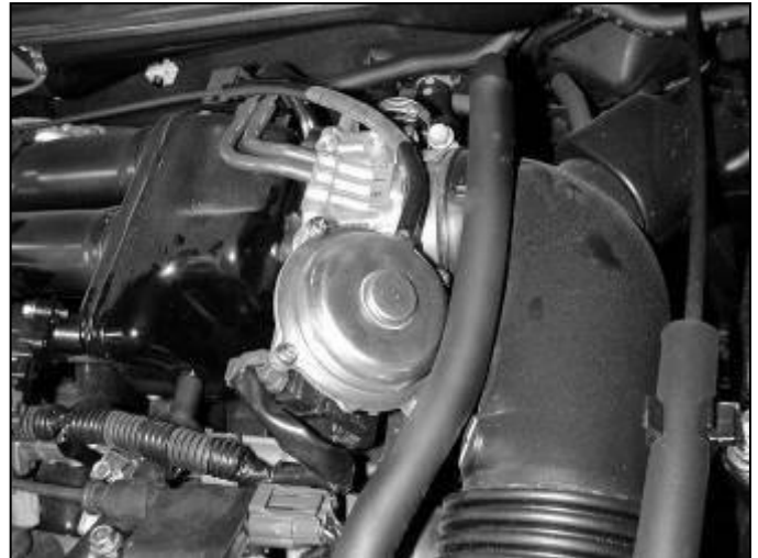
b. Pull breather hose off of valve cover. Loosen the upper and lower hose clamps on the stock inlet tube.
