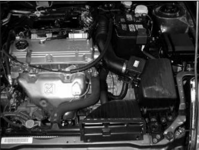
a. Stock air box system installed.
