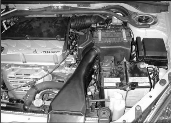
Factory air box system installed
