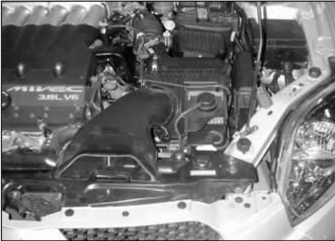
Factory airbox system installed
