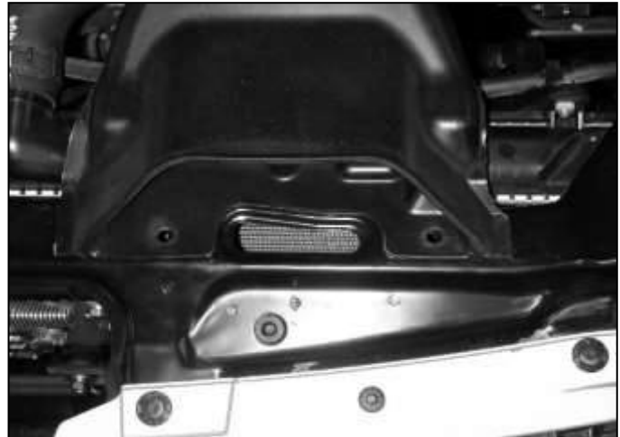
b. Remove the 2 plastic rivets securing the intake duct to the radiator support.
