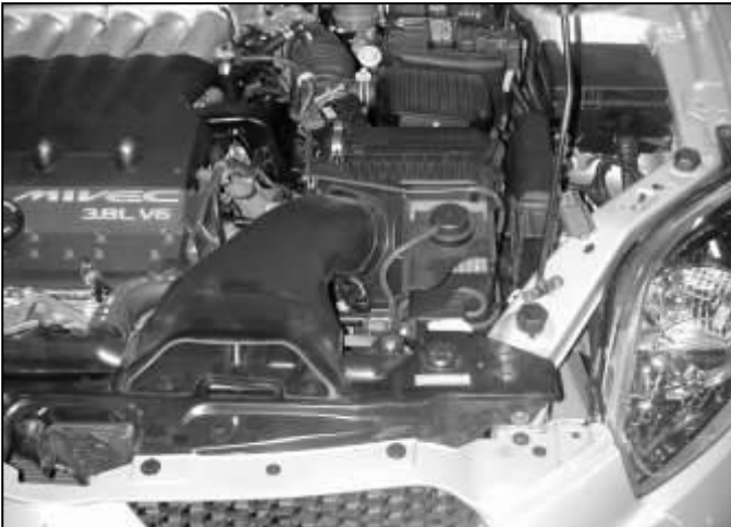
a. Factory airbox system installed.
