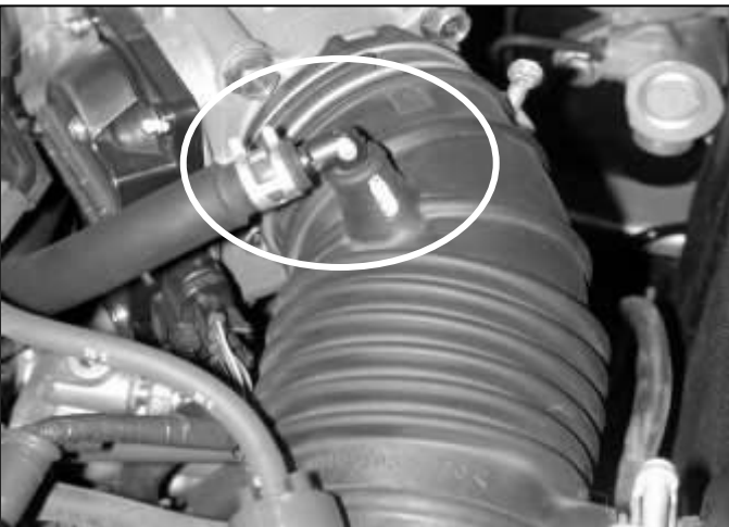
c. Remove the breather hose from the inlet air tube by compressing the spring clamp and pulling it off.
