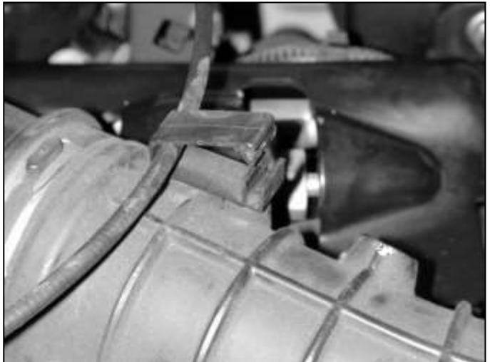
b. Release the clip on top of the inlet pipe.
