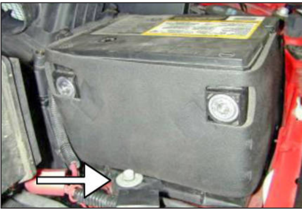
g. Loosen the battery hold down bolt and remove the battery.
