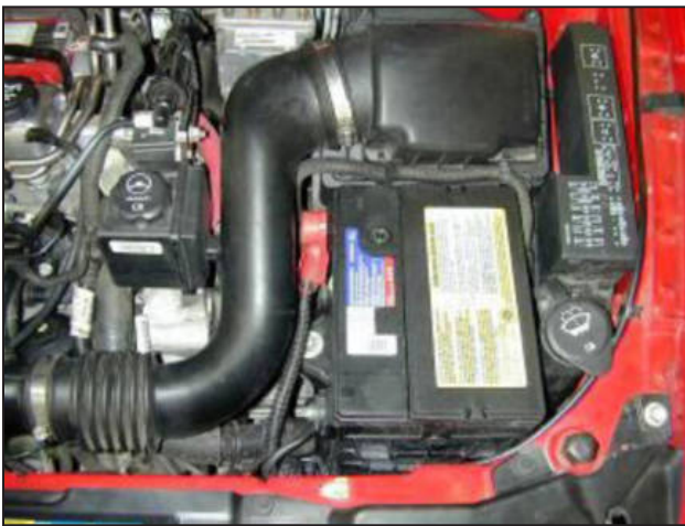
a. Stock air box system installed.
