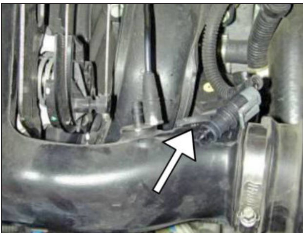
c. Pull the vacuum hose off of the inlet pipe, if equipped. Pull the IAT sensor out of the pipe. Remove the rubber grommet and save for later use.
