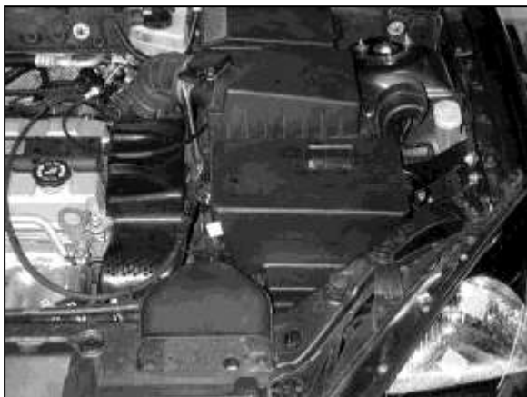
a. Factory air box system installed.
