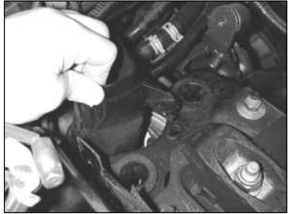
l. Remove the lower intake pipe tab from the grommet hole.
