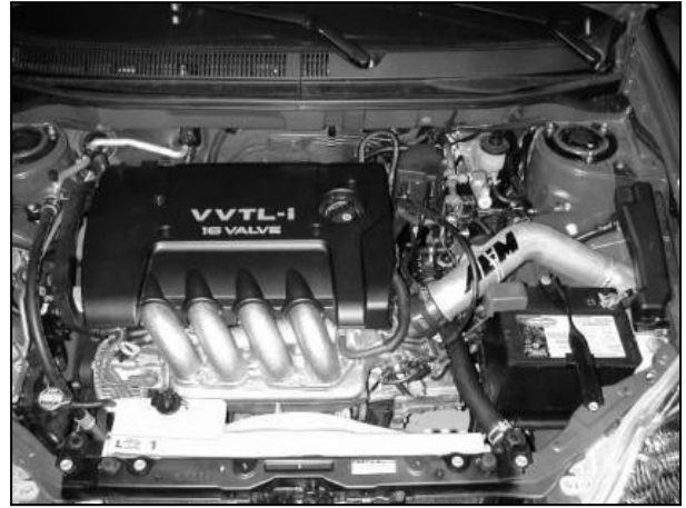
AEM ® intake system installed
