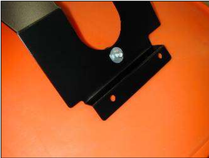
f. Secure rubber mount with washer and Nylok nut. Place the intake into the cavity left by the air box filter first.
