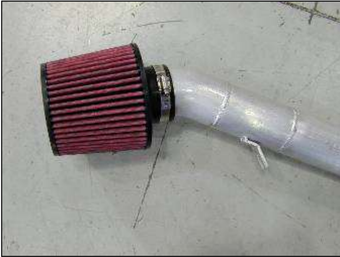
d. Attach the air filter and tighten.
