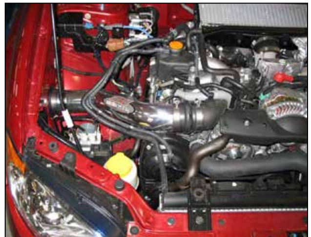
AEM® intake system installed
