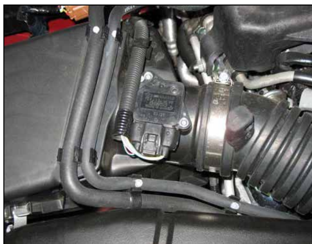
b. Unplug the mass air flow sensor (MAF) wiring harness.
