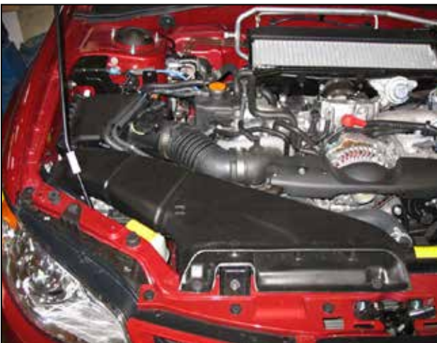
Stock air box system installed
