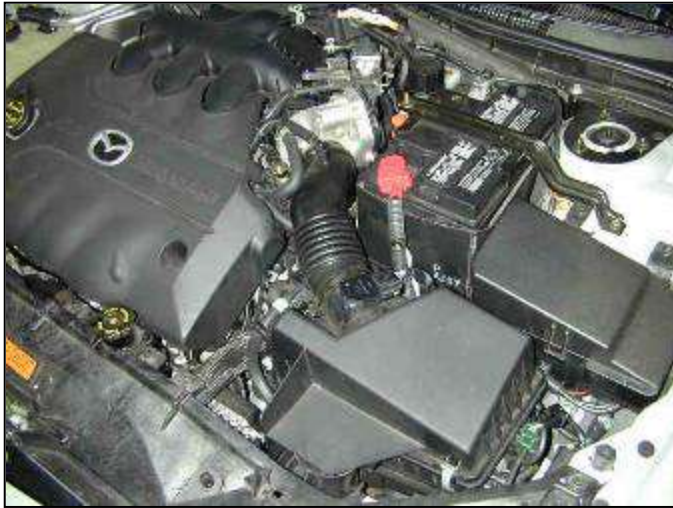
a. Stock air box system installed.
