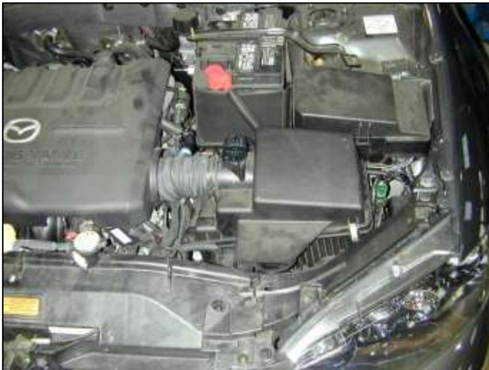
Factory air box system installed
