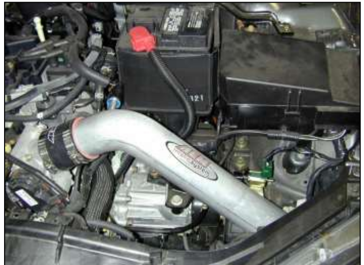
AEM® intake system installed
