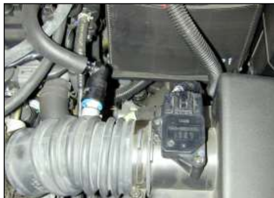
c. Unplug the MAF sensor from the wiring harness. Unclip the wiring harness from the back of the air filter housing.
