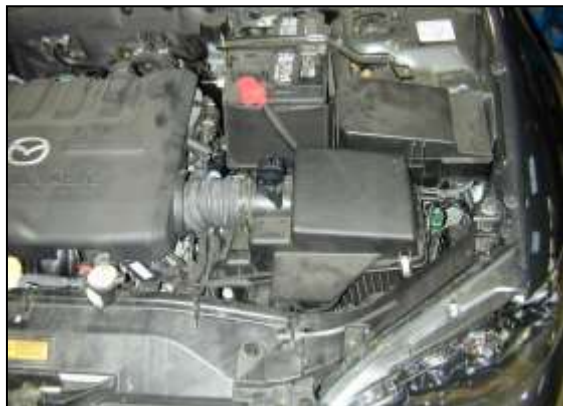
a. Factory air box system installed.
