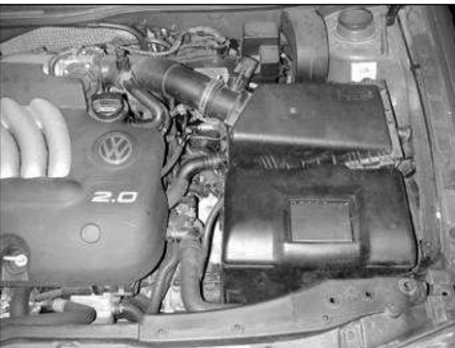
Factory airbox system installed
