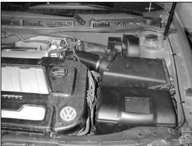
Factory air box system installed
