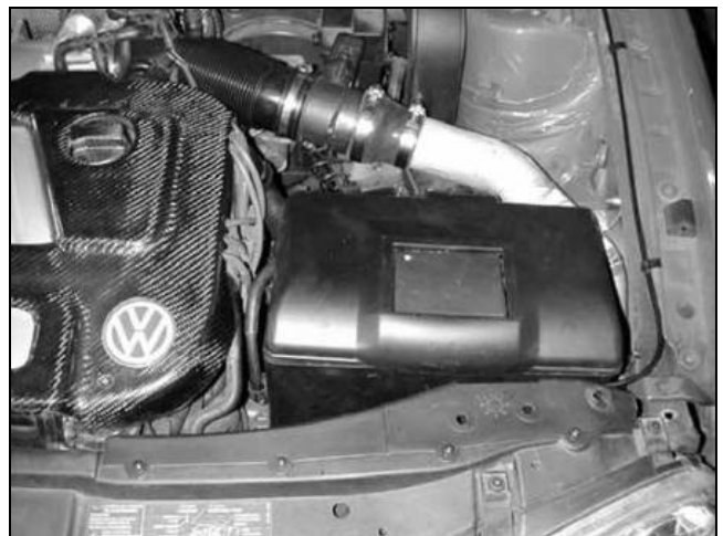
AEM® intake system installed
