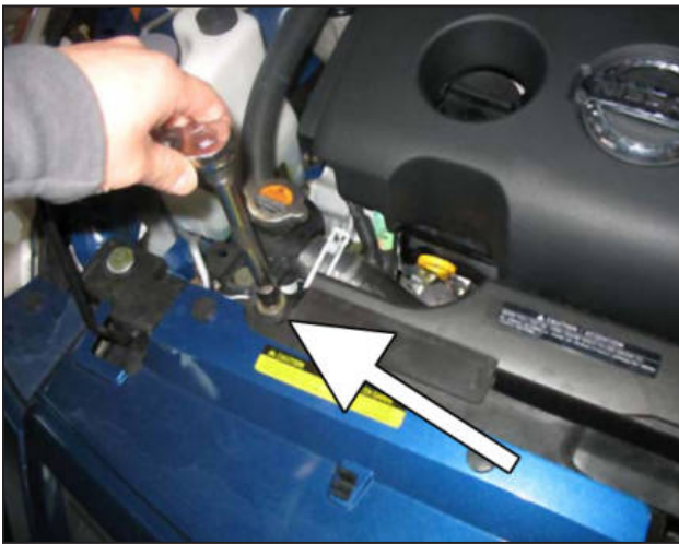
c. Loosen and remove the hex head screw on the trim cover.
