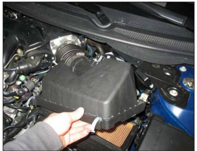
n. Remove the air box lid and the inlet duct.
