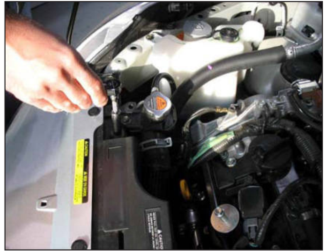
ag. Using the factory hex head bolt, secure the radiator trim panel in place.
