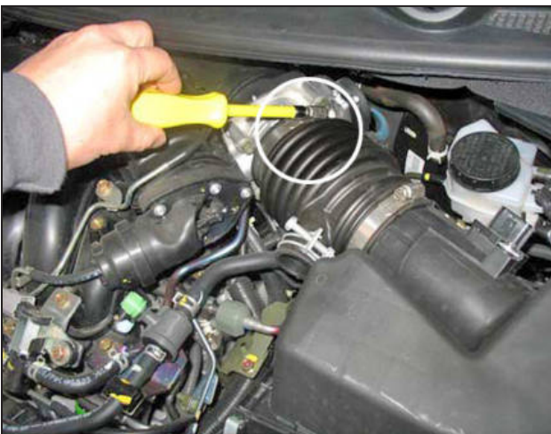
i. Loosen the hose clamp securing the inlet duct to the throttle body.
