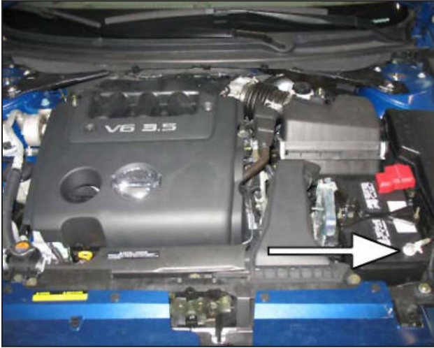
a. Open the hood and disconnect the negative battery cable.
