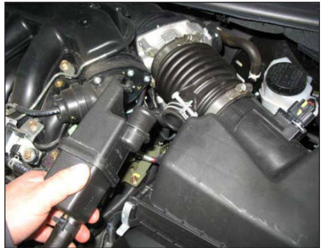
h. Remove the PCV resonator from the inlet duct.
