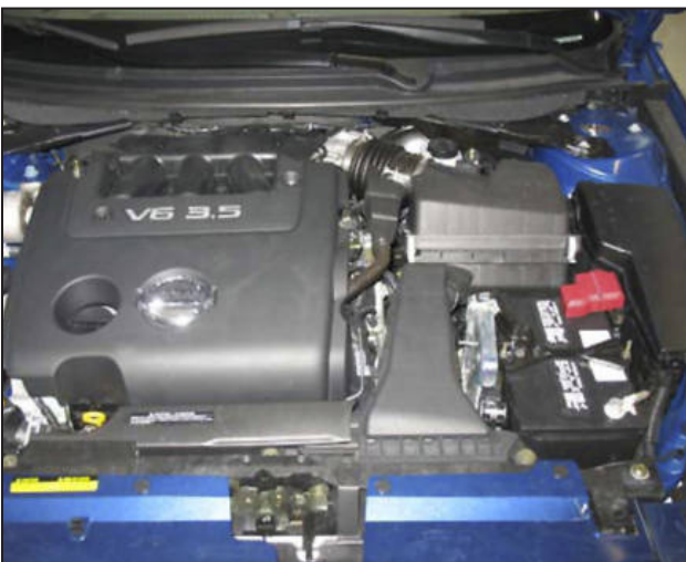
Factory air box system installed
