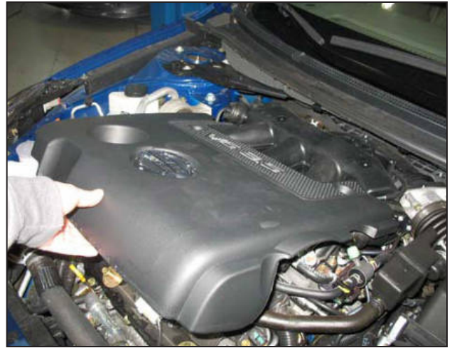
f. Remove the engine cover by pulling the cover upward at the front edge.
