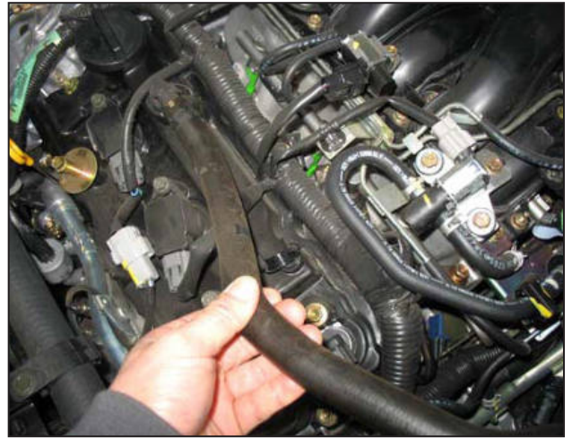
l. Remove the PCV hose from the vehicle.
