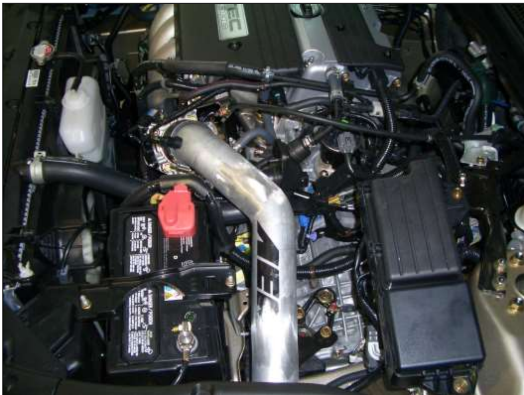
AEM® intake system installed
