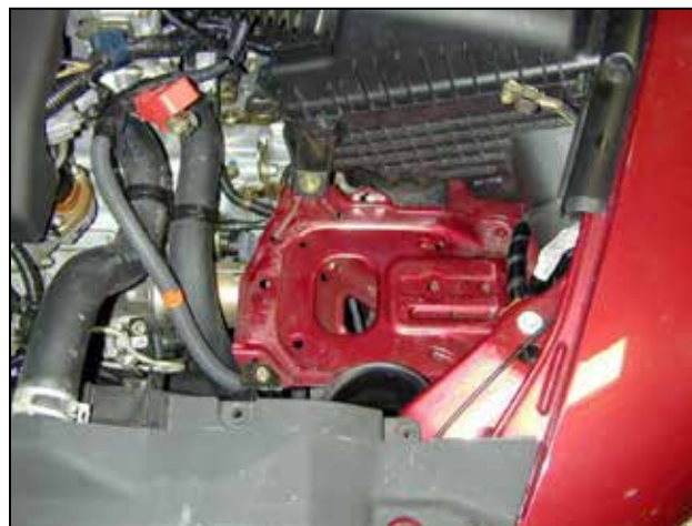
d. Unclip the plastic battery shroud from the positive terminal wire and remove the shroud.
