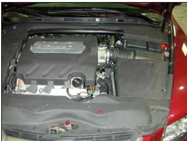
a. Factory air box system installed.
