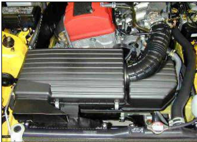
Factory air box system installed
