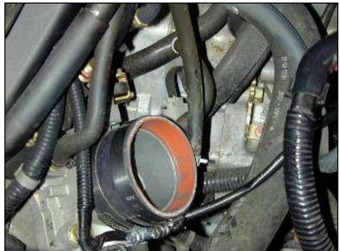
e. Attach the coupler to the throttle body with hose clamps as shown. Tighten only the clamp on the throttle body.
