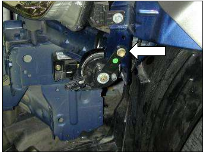
c. Remove 8mm bolt that secures the horn to the chassis. NOTE: The horn sits inward toward the chassis.
