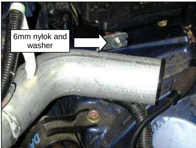
h. Secure bracket to rubber mount with 6mm washer and nylok nut and tighten. Refer to diagram below for proper rubber mount installation.
