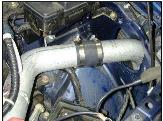
i. Install lower pipe from below, up through the frame rail hole and into coupler. Push the pipe all the way together. Do not fully tighten clamps.
