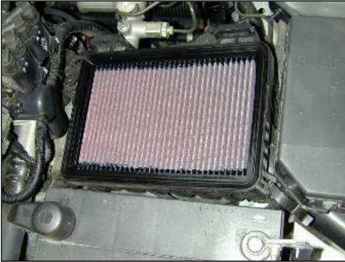
c. Remove the air filter element to gain access to lower air box mounting hardware.
