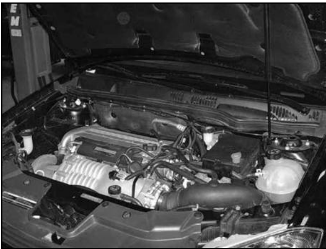
a. Factory air box system installed.
