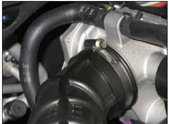
d. Loosen the hose clamp on the throttle body.
