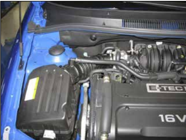
a. Stock air box system installed.
