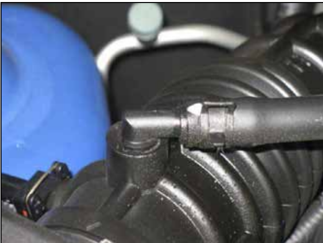
c. Remove the breather hose from the inlet tube.
