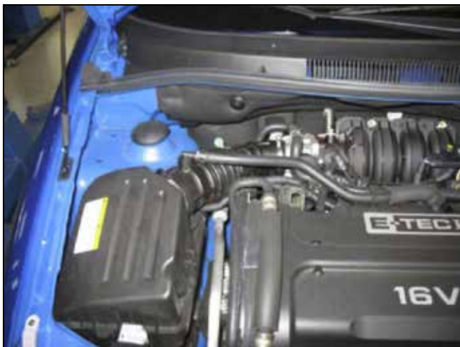
Stock air box system installed.
