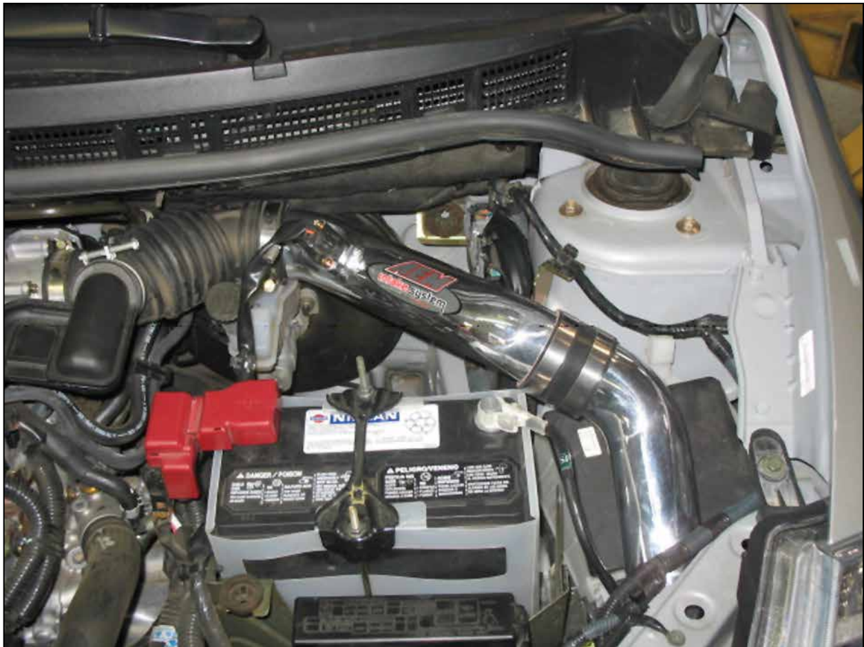
AEM® intake system installed
