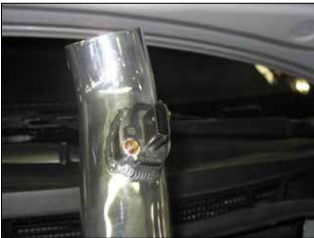
f. Reinstall the MAF Sensor with factory bolts into the AEM® inlet pipe.
