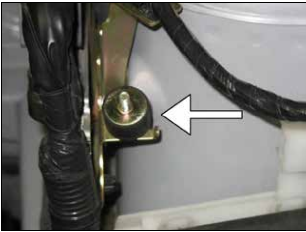
d. Install the 5/8" rubber mount into the ECU bracket.
