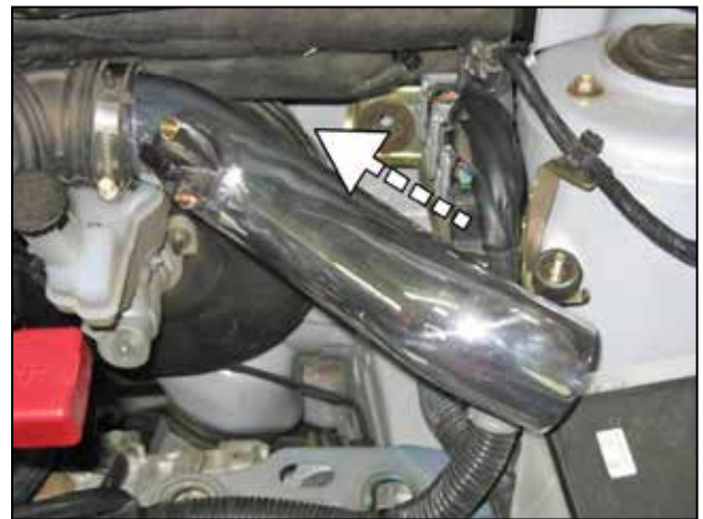
g. Insert the inlet pipe as shown.
