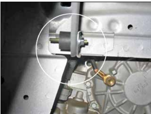
h. Attach the 1" rubber mount in the fender well. Secure the backside of the rubber mount with the M6 washer and M6 Nut.
