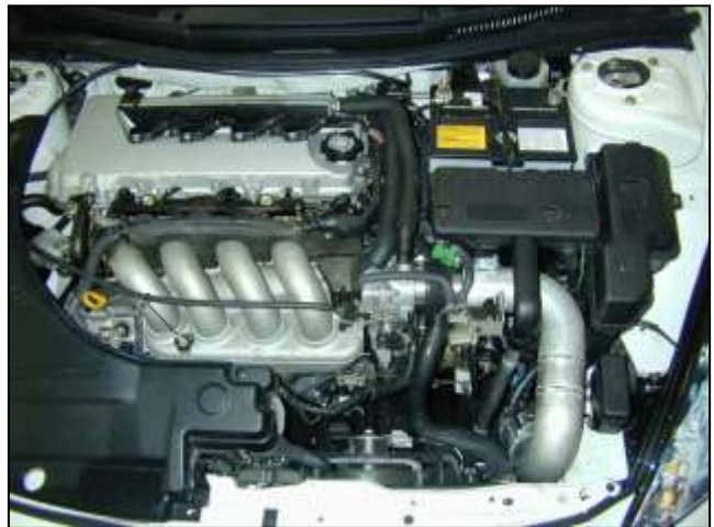
AEM ® intake system installed.
