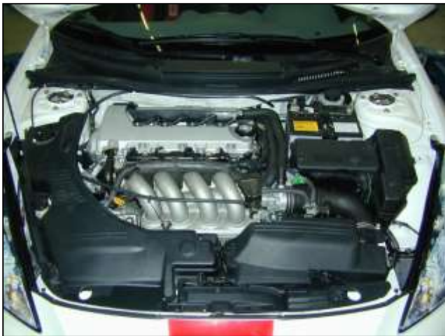
Stock air box system installed
