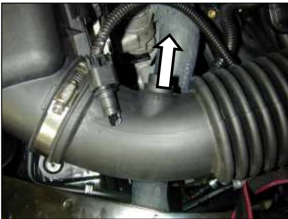
e. Gently pull out the inlet air temp (IAT) sensor from the rubber grommet.
