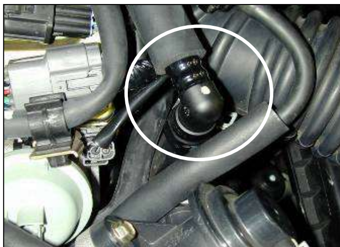
b. Disconnect the plastic breather hose from the inlet tube. This is done by squeezing the blue retaining clip and pulling on the breather hose.
