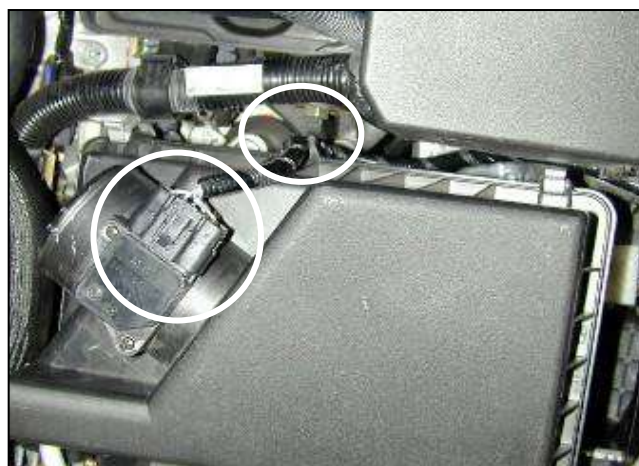
d. Disconnect the MAF sensor wiring harness from the sensor and unclip it from the side of the air box.
