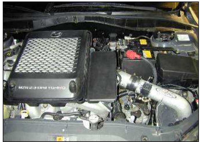
AEM® intake system installed
