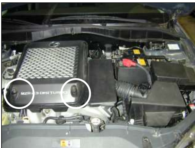
a. Remove plastic intercooler cover by removing the 2 bolts securing it to the intake manifold.
