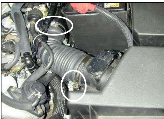
c. Loosen the hose clamps securing the inlet hose to the stock air box and turbo inlet pipe. Remove the inlet hose.
