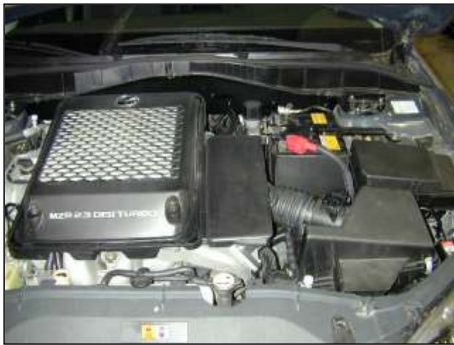
Factory air box system installed
