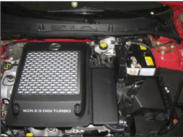
Factory air box system installed
