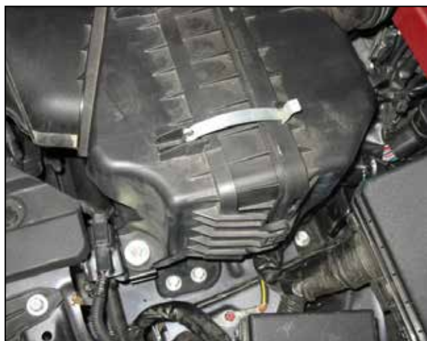
d. Remove the bolt securing the OE air box to the vehicle.
