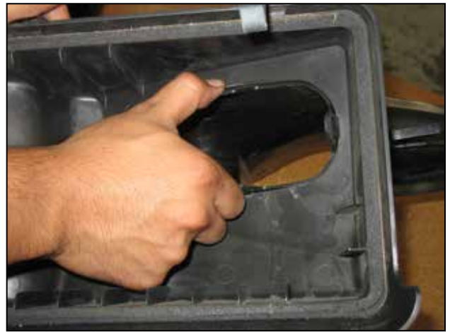
t. Separate the air box housing, then remove the inlet duct from the air box by squeezing the top two tabs and pushing out.
