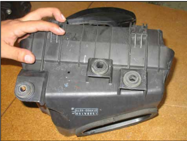
u. Remove the two grommets on the bottom of the air box housing. They will be reused in a later step during the AEM® intake system installation.
