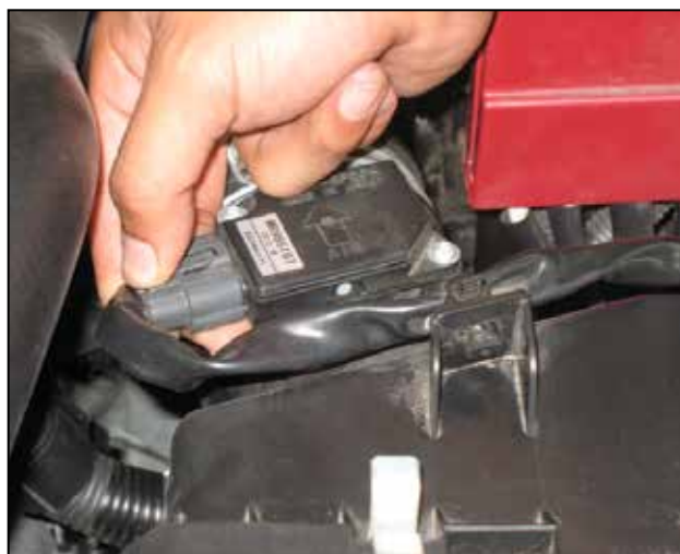
b. Disconnect the mass air flow (MAF) sensor harness connector from the MAF sensor.
