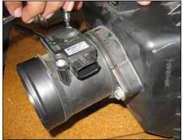
r. Remove the MAF sensor from the air box housing using the supplied tamper proof torx tool.
