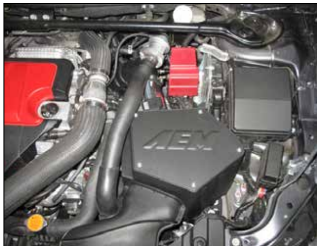
AEM® intake system installed
