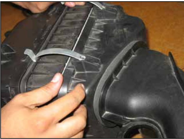
s. Unclip the two clips holding the air box housing together.
