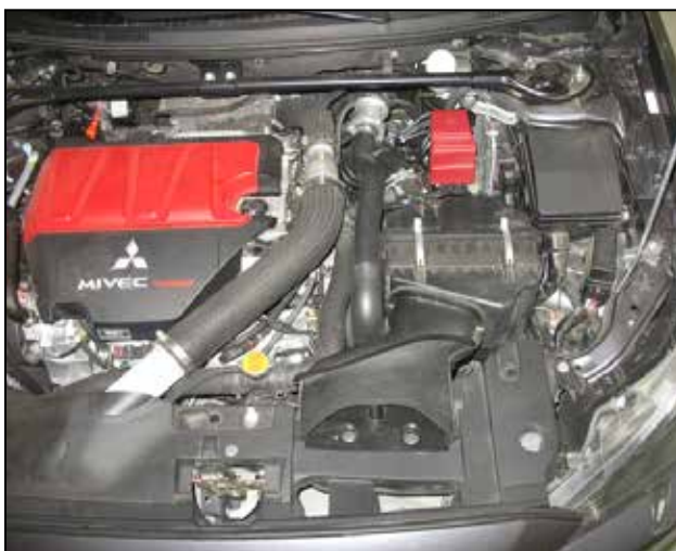
a. Stock air box system installed.
