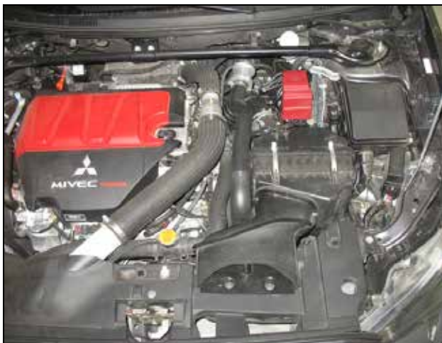
Factory air box system installed
