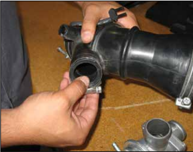
q. Remove the hose clamp from the inlet tube.
