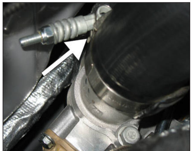
j. Loosen the t-bolt clamp in the direction as indicated in the photo.
