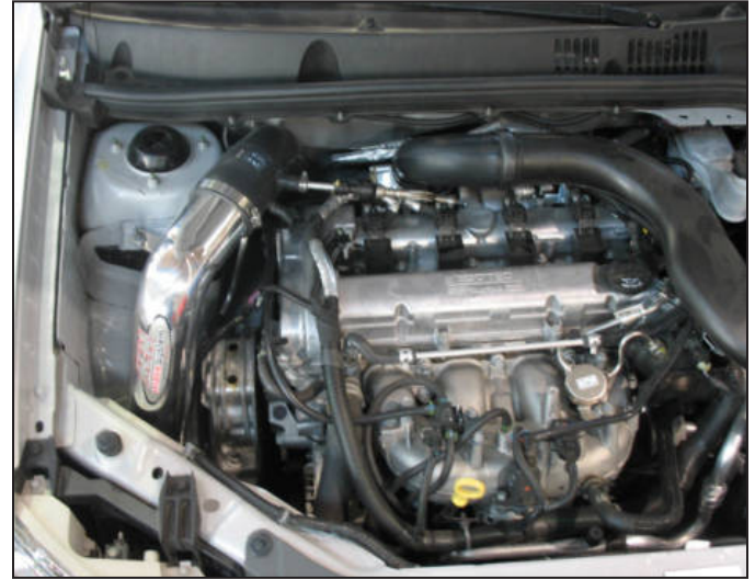
AEM® intake system installed
