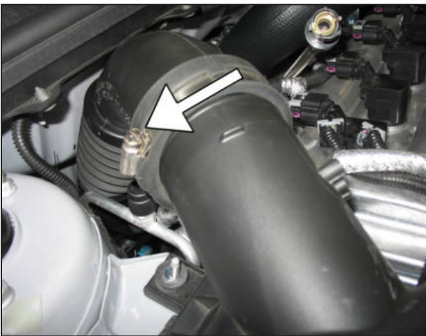
g. Using an 8mm nut driver, loosen the hose clamp as shown.
