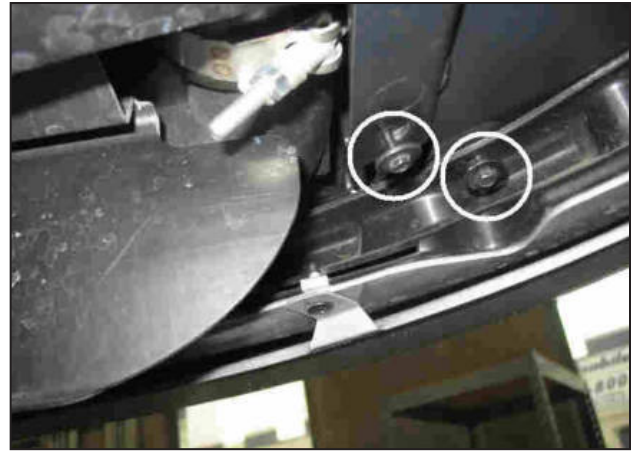
n. Remove the additional 7mm bolts and push clips on the corresponding bottom section.
