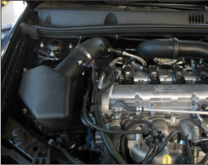
Stock air box system installed
