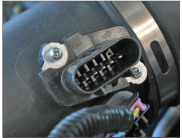
f. Remove the MAF sensor from the inlet tube with a philips screwdriver.
