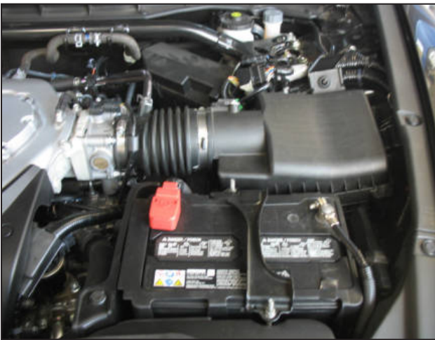
a. Stock air box system installed.
