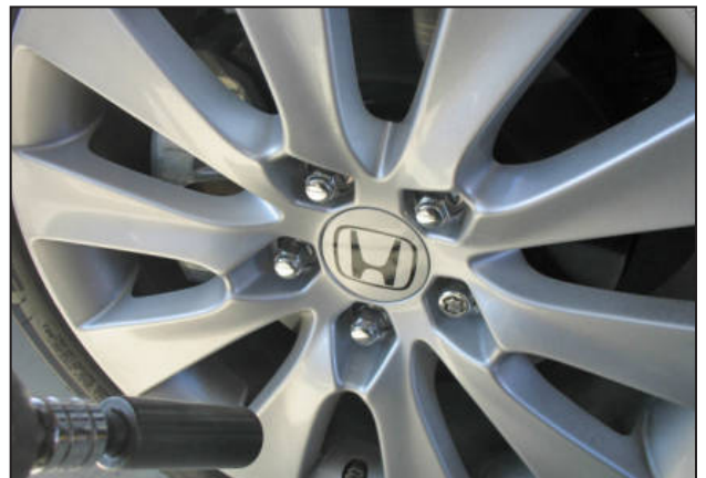
o. Raise the front of the vehicle with a jack. Refer to your owner's manual for proper jack and jack stand placement to properly support vehicle. Support your vehicle using properly rated jack stands before wheel removal or while working under the vehicle. NEVER WORK UNDER A VEHICLE WITHOUT USING JACK STANDS. Remove the driver-side front wheel with a 19mm socket.
