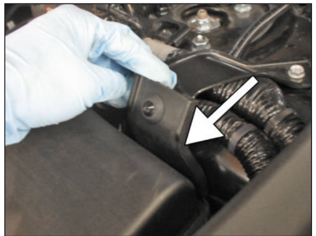
m. Push the air box panel unit out from the dowel and set aside.
