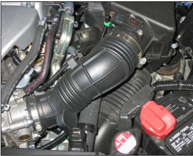
a. Stock air box system installed.
