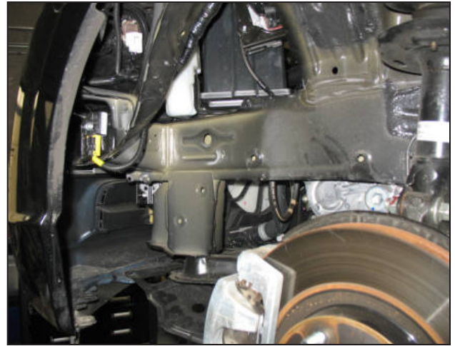
s. Stock air box system removed from the vehicle.
