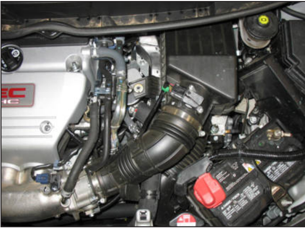
Factory air box system installed
