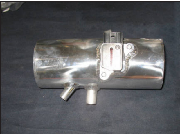
b. Carefully install the MAF sensor into the upper intake pipe using the two stock bolts.
