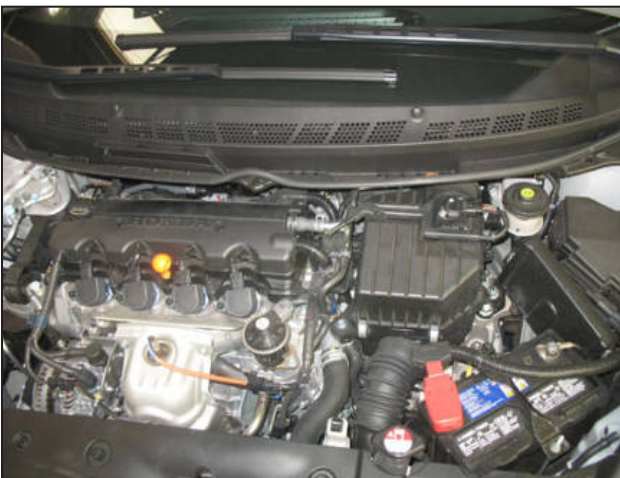
Stock air box system installed
