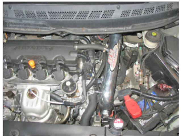
AEM® intake system installed
