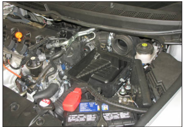
h. Remove the stock panel air filter.
