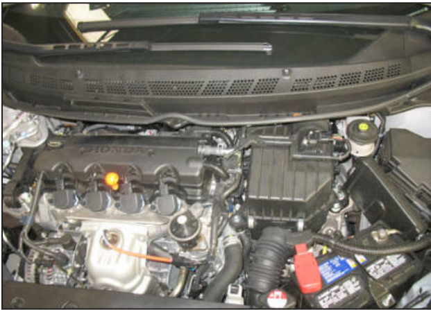
a. Stock air box system installed.
