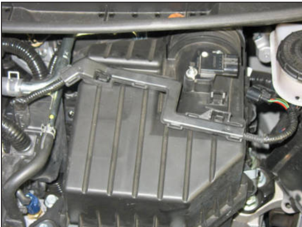
c. Remove the wire harness from the clips located on the air box lid.
