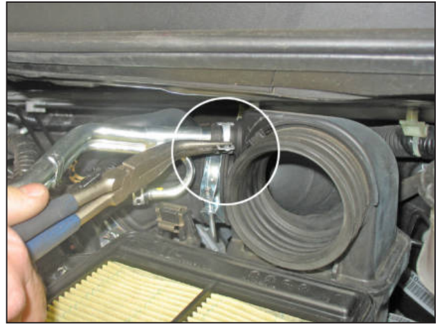
f. Disconnect the PCV hard line from the rubber inlet.
