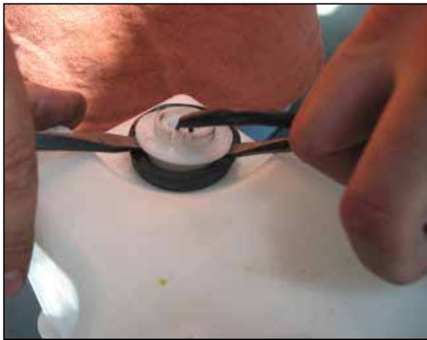
l. Using two flat head screwdrivers, carefully pry up on the lip of the washer level sensor. Take care not to damage the rubber grommet. Some liquid soap and water mixture applied to the sensor may help with removal. Also remove the grommet and set it aside.
