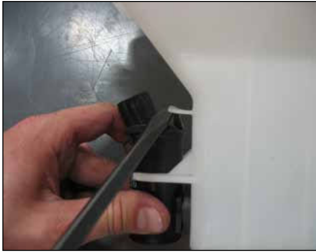
j. Using a flat head screwdriver, unclip the washer pump from the washer bottle as shown.
