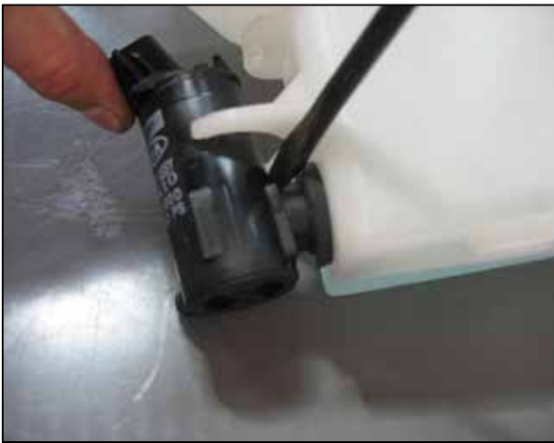
k. Pry the washer pump out of the grommet and set it aside. Also remove the grommet and set it aside.
