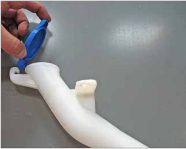
i. Remove the blue washer fluid cap from the washer bottle neck by carefully unsnapping it from the neck.
