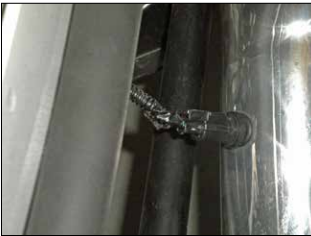
v. Plug the IAT sensor harness connector back onto the IAT sensor.
