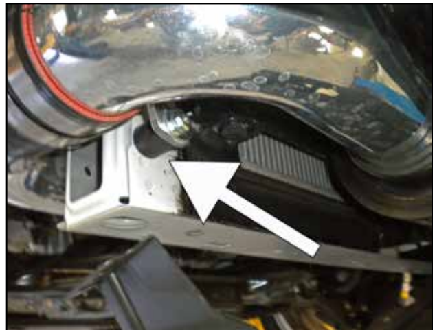
s. Secure with a washer and nut.
