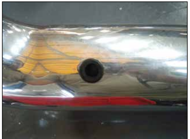
e. Install the grommet in the middle pipe.
