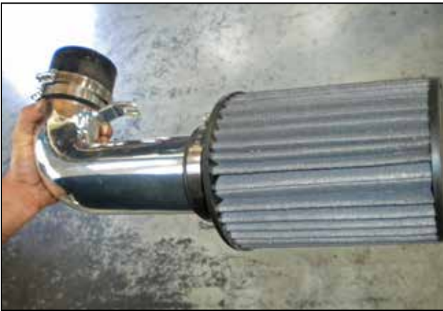
p. Install the air filter on the lower pipe.
