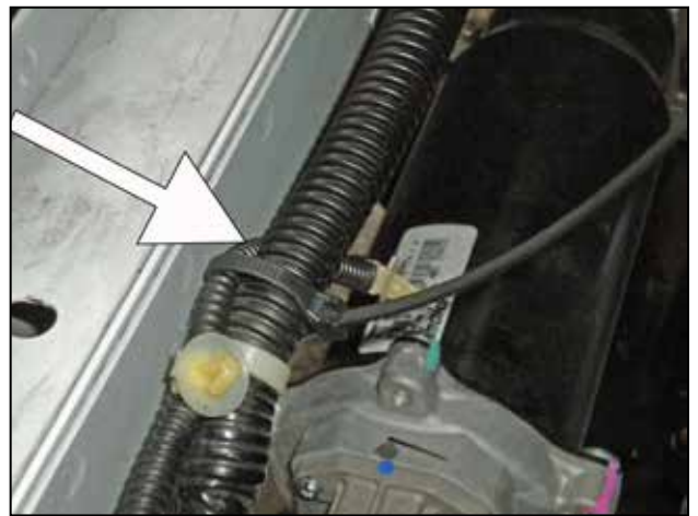
w. Zip tie the IAT harness to the large wire harness located on the frame rail.
