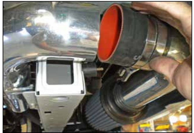
q. Connect the lower pipe to the middle pipe.
