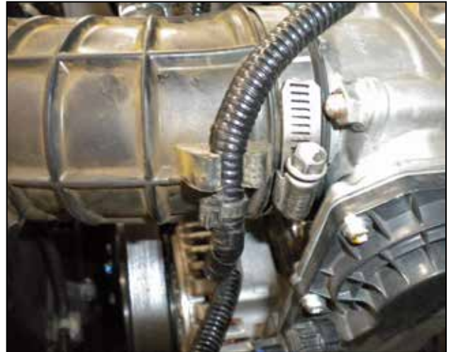
b. Remove the wire harness connected to the inlet tube.
