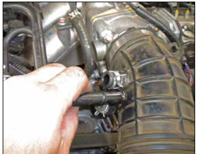
j. Disconnect the PCV hard line from the inlet tube.
