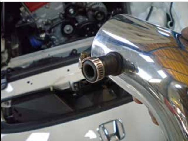
d. Loosely install the hose clamp on the PCV adapter.
