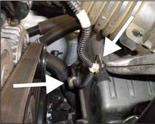
k. Disconnect the zip tie securing the IAT harness to the air box.
