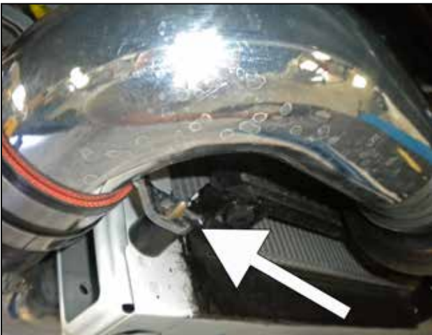
r. Align the lower pipe bracket with the rubber mount as shown.
