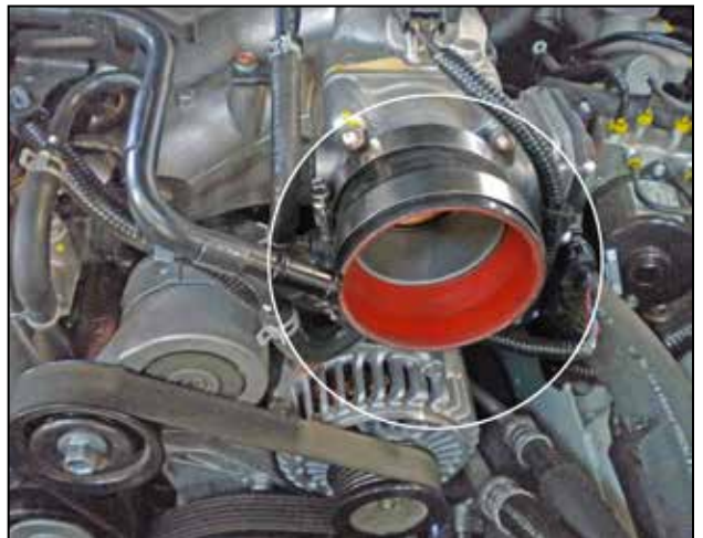
g. Install the reducer coupler with the hose clamps onto the throttle body.
