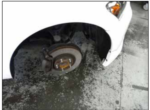
n. Remove passenger side wheel.
