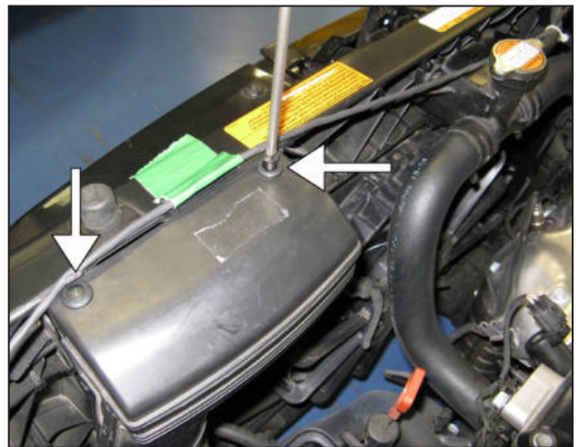
h. Remove 2 Phillips screws mounting the bypass pipe to the radiator top support frame rail.
