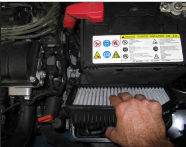
g. Remove the original air filter from the lower housing.
