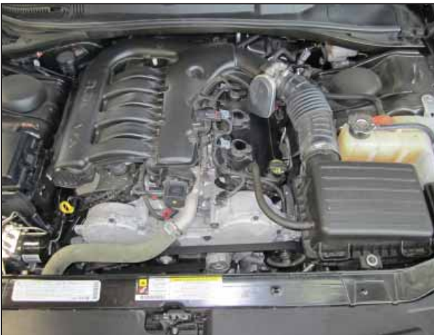
Stock air box system installed
