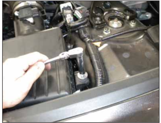
l. Loosen and remove the 10mm bolt at the top of the air box.
