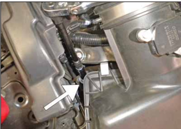
m. Remove the 10mm bolt located at the bottom of the air box.
