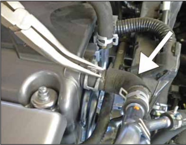
k. Release the spring clamp and remove the PCV hose from the valve cover.
