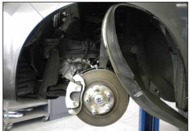
p. Remove the clips securing the fender liner and partially remove the fender liner as shown.
