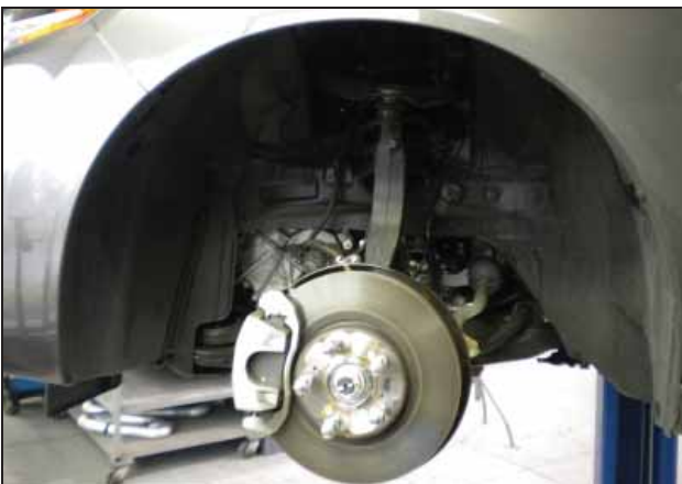
o. Raise the front of the vehicle with a jack. Refer to your owner's manual for proper jack and jack stand placement to properly support vehicle. Support your vehicle using properly rated jack stands before wheel removal or while working under the vehicle. NEVER WORK UNDER A VEHICLE WITHOUT USING JACK STANDS. Remove the driver side front wheel.
