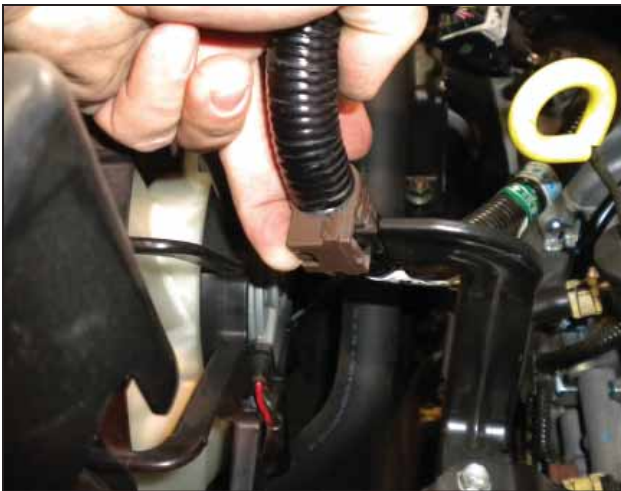
c. Disconnect the power wire clip.
