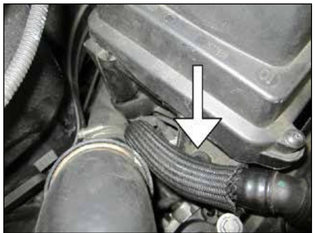
d. Remove the lower Torx screw and plastic grommet insert at the passenger side foot of the stock air box using a T20 Torx bit. Retain the Torx screw for future use.
