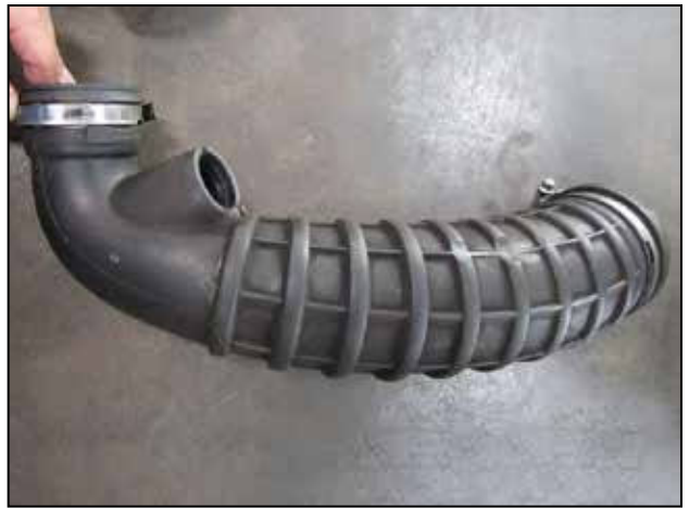
b. To remove the stock intake tube, disconnect the turbo bypass tube from the stock intake and loosen the 2 hose clamps retaining the intake tube.
