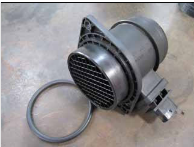
c. To remove the stock MAF sensor housing, remove the 2 screws retaining the MAF housing to the upper air box lid, then remove the large o-ring from the MAF sensor outlet.
