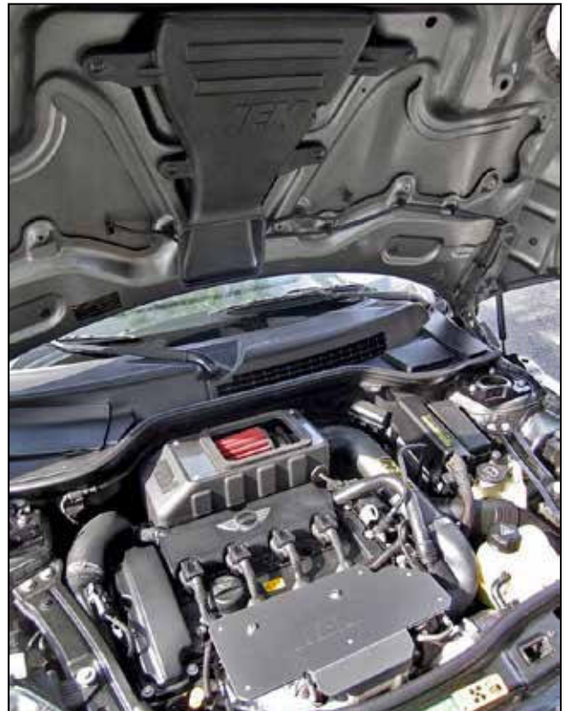
AEM® intake system installed
