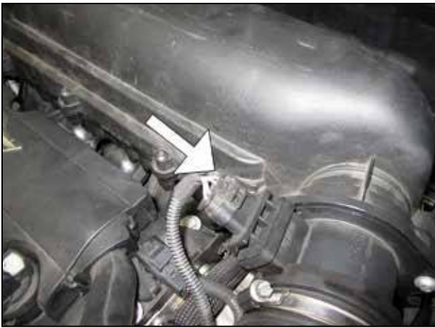
a. Disconnect the MAF sensor wiring harness at the MAF sensor housing by pushing down the small lock tab and pulling on the connector.
