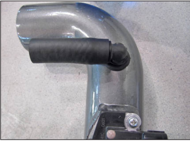
f. Insert the 90° fitting assembly into the grommet as shown.
