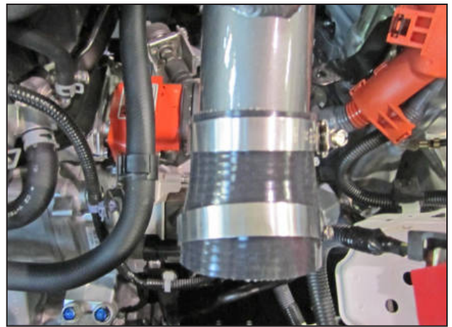
i. Install a reducer coupler (#5-255) onto the end of the upper intake pipe and secure with hose clamp (#9436). Slide hose clamp (9440) onto the open end of the coupler as shown.
