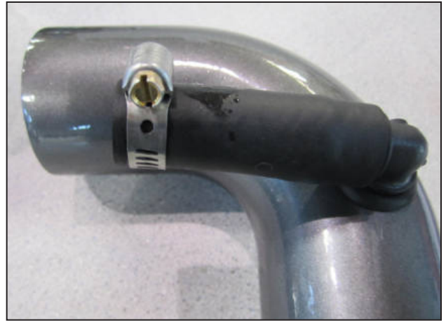
g. Slide hose clamp (4093-5) onto the hose as shown.
