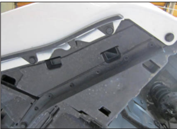
m. Remove the 4 clips securing the fender liner to the bottom of the front bumper.
