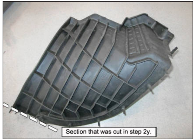
z. Remove the section of the rubber valence that was cut free in the previous step.
