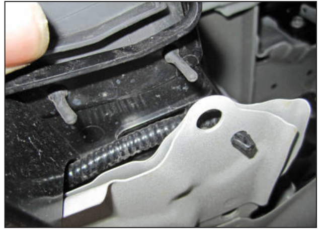
x. The rubber valence needs to be trimmed on the driver side. Separate the rubber piece from the hard plastic piece by pulling on the rubber portion until the nipples disengage the plastic side of the valence.
