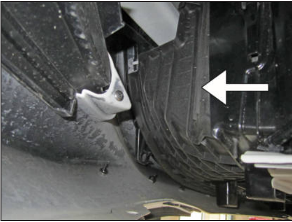
w. From underneath the vehicle, locate the rubber valence on the driver side behind the front bumper.
