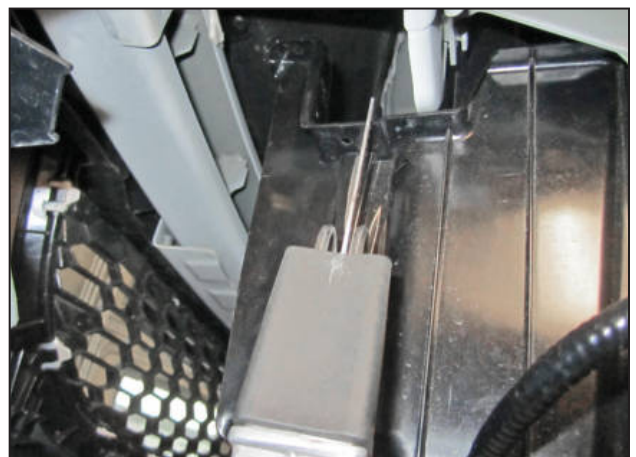
ab. Trim the valence along the mark, marked in the previous step.
