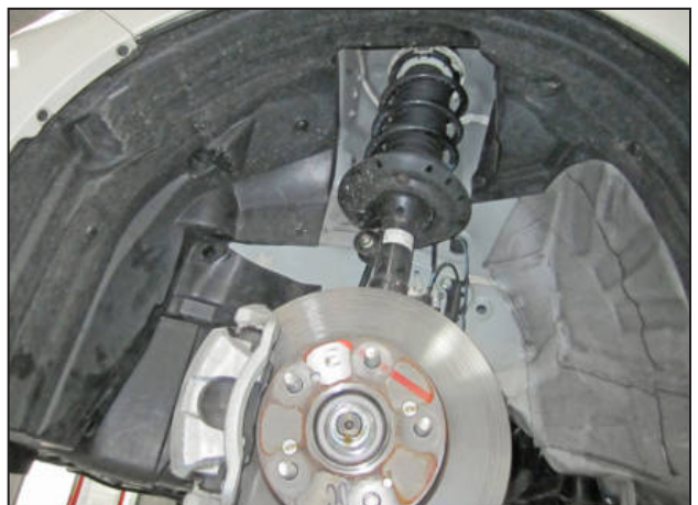
p. Remove the 9 clips securing the fender liner to the fender well.
