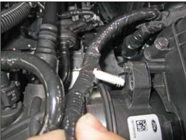
c. Unplug the wire harness clip securing the harness to the MAF sensor bracket.
