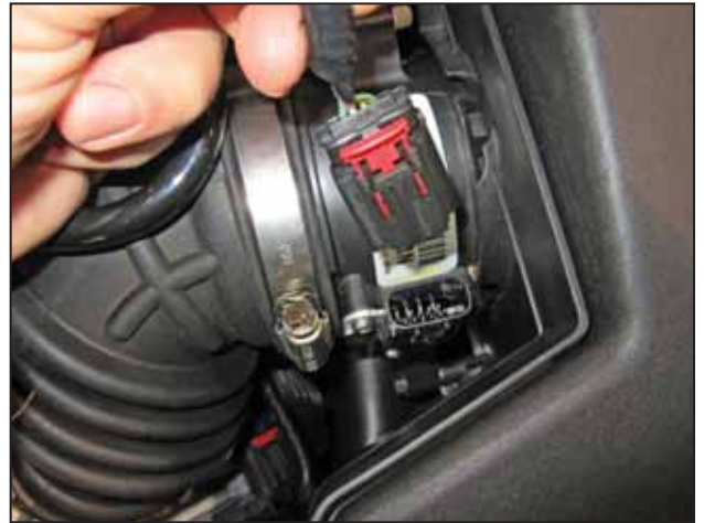
b. Lift up on the red locking clip and unplug the MAF sensor.
