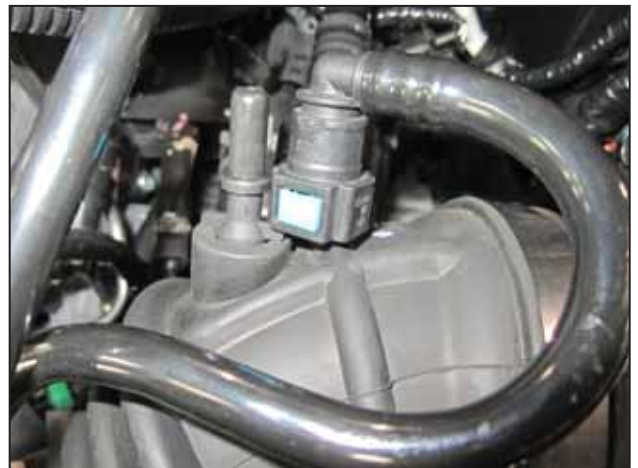
d. Locate PCV hose #1 (Blue locking mechanism) at the top of the intake tube and disconnect the connection as shown.
