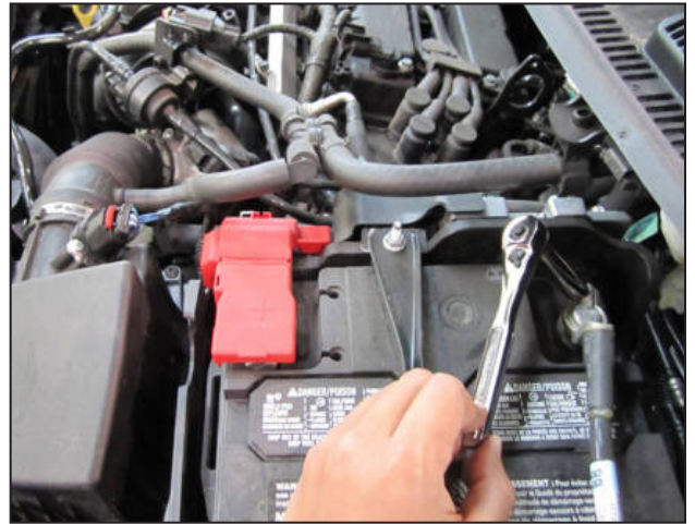
b. Disconnect the negative battery terminal using a 10mm socket. Also disconnect the MAF sensor harness connector from the MAF sensor.
