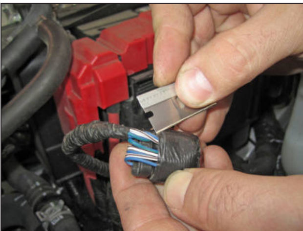
c. Remove the electrical tape from the MAF sensor clip.
