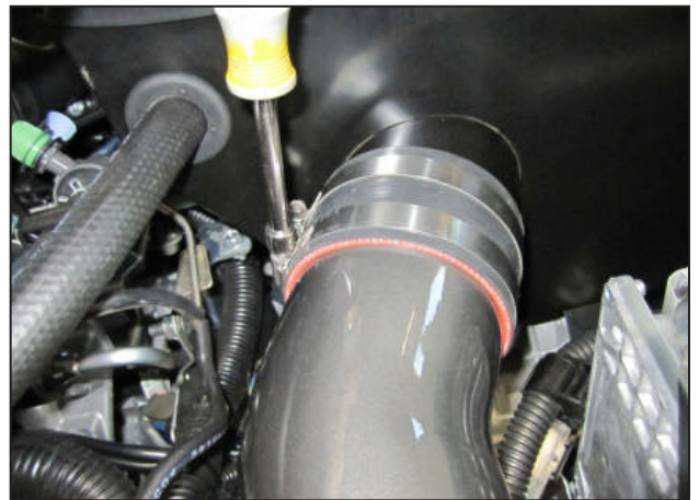
am. Tighten the hose clamp securing the air intake tube to the heat shield inlet.
