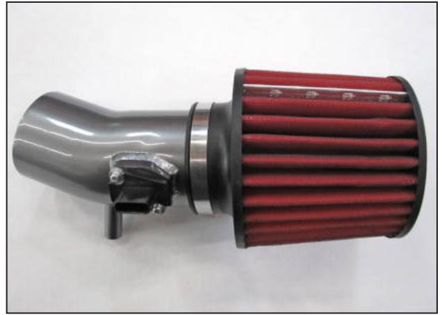
ae. Mount the AEM® air filter onto the intake tube and secure using a #56 hose clamp.
