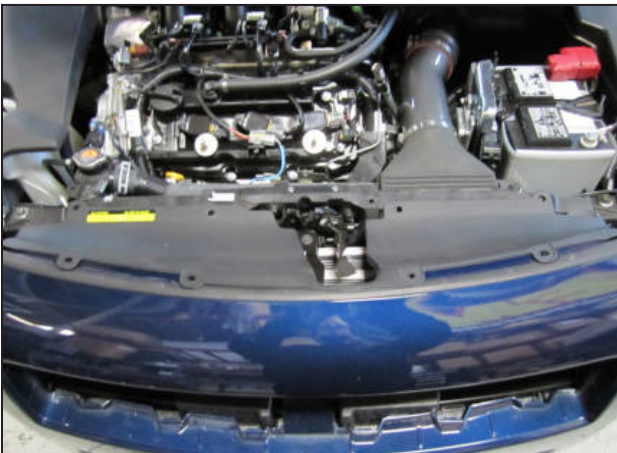
an. Reinstall the radiator shroud.
