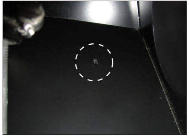
ak. Once the transmission breather hose clip is properly secured to the heat shield hole, it should look like this.
