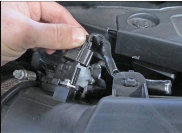
g. Unplug the MAF sensor connector.
