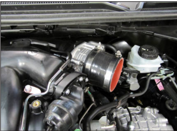
b. Install coupler (5-325) onto the throttle body and mount two #52 hose clamps as shown.
