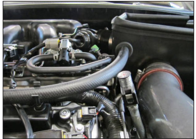
ac. Feed the PCV vent hose through the heat shield hole as shown.
