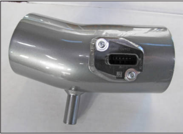
ad. Install the MAF sensor onto the intake tube (2-1481) using the OEM screws.
