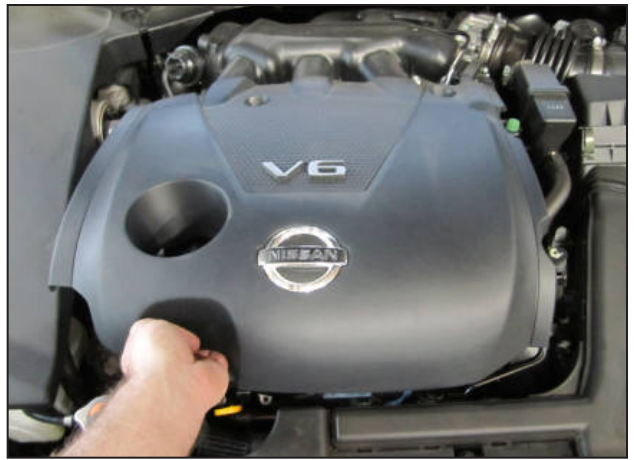
b. Lift up on the bottom of the engine cover and remove from the vehicle.
