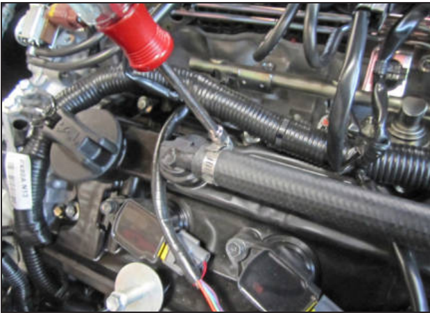
ab. Attach the provided vent hose (5-7021) to the PCV port on the valve cover and secure with a hose clamp (08411).
