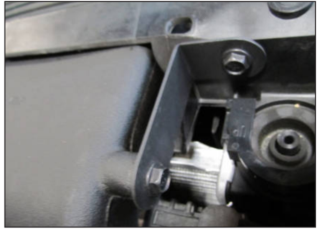
y. Secure the air inlet scoop's bracket to the radiator support using one M6 bolt (1-2110).
