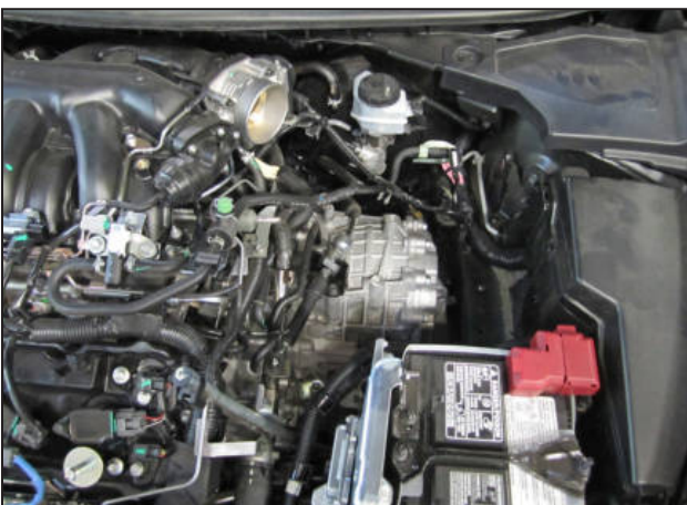
o. Remove the factory air box system from the vehicle.
