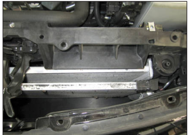
t. Remove the shroud from the vehicle.
