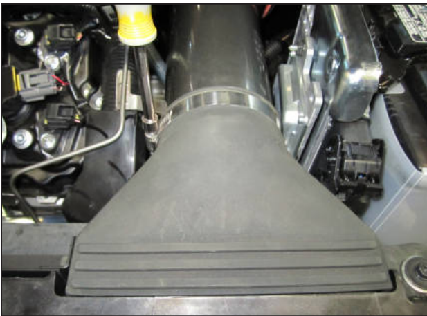
al. Tighten the hose clamp securing the air inlet hose to the air intake tube.
