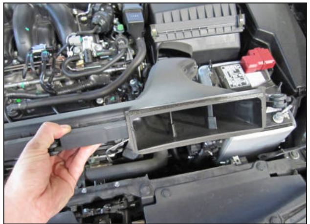
d. Remove the stock intake scoop from the vehicle.
