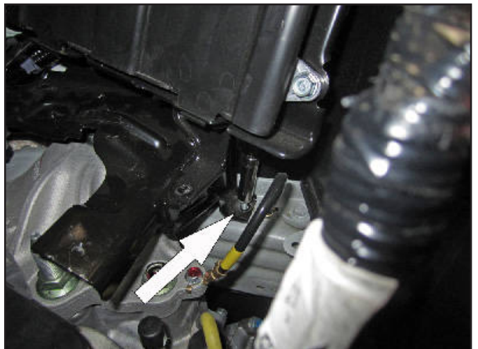
l. Remove the lower 10mm bracket bolt.
