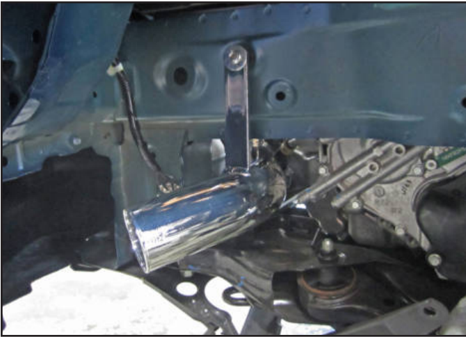
l. Install the lower intake tube.
