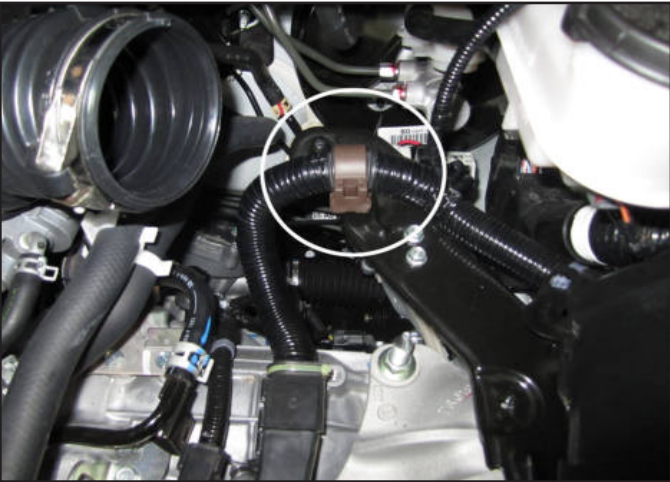
q. Reinstall the bracket back into the engine compartment, moving the wire harness on top of the bracket.
