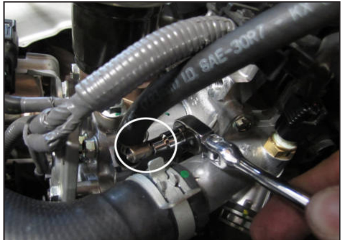
c. Tighten the 1/4" hose clamp on the engine inlet as shown.
