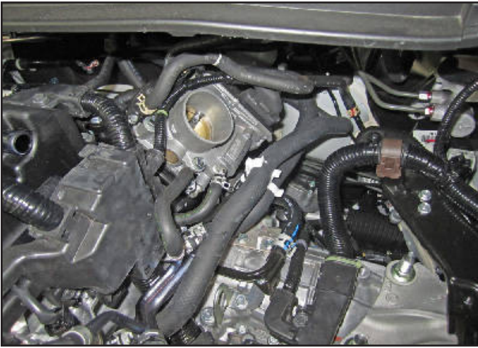
u. Remove the stock intake tube from the vehicle's engine compartment.
