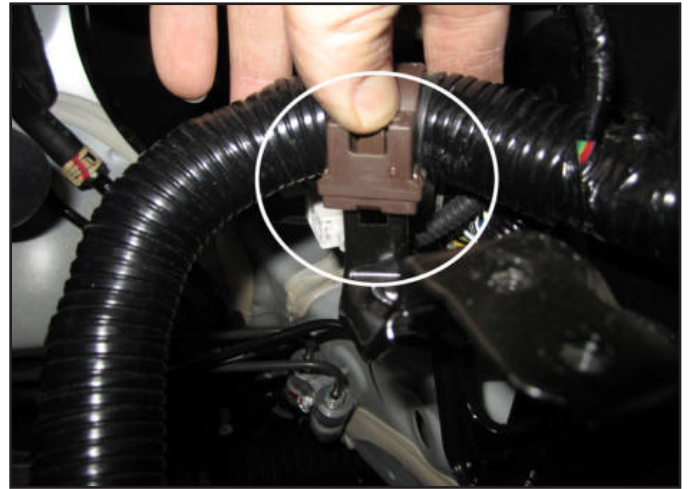
p. Release the wire harness clip from the bracket.
