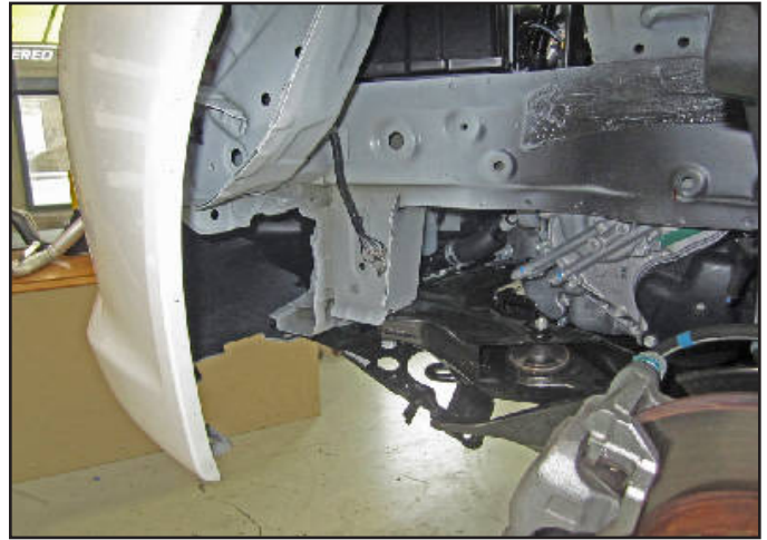
ab. Remove the resonator tube.
