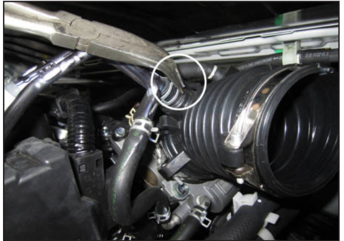
r. Release the clip on the PCV pipe and remove the pipe from the intake tube.
