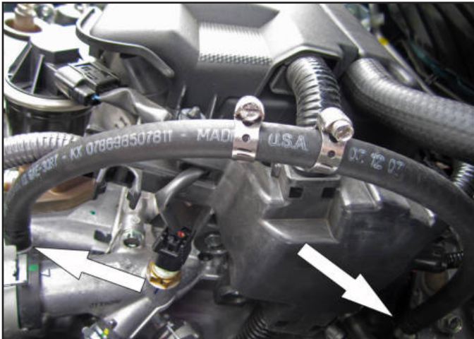
b. Install the provided 5/16" coolant hose and clamps onto the engine inlet and the throttle body inlet.
