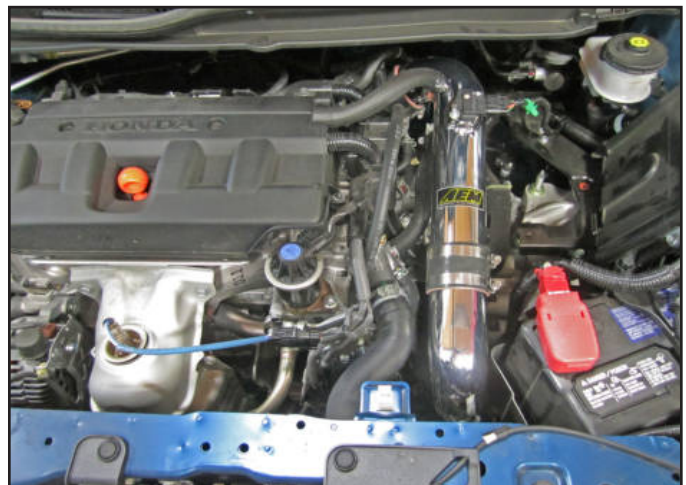
AEM® intake system installed.
