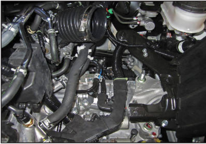
i. Remove the air box from the vehicle's engine compartment.
