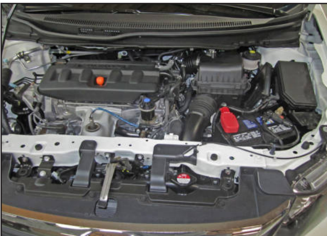
Stock air box system installed.
