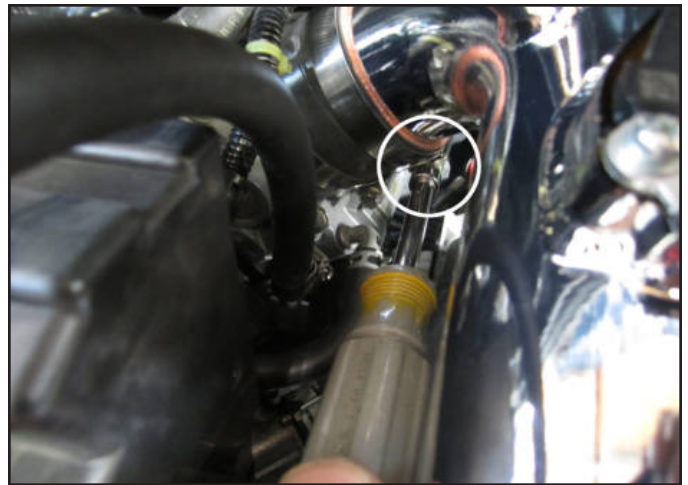
o. Align and adjust the upper intake tube for clearance, then tighten the hose clamp on the throttle body.
