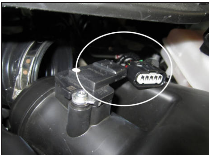
g. Disconnect the mass air flow sensor.
