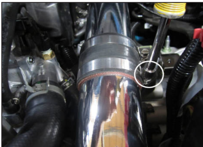
p. Tighten the hose clamp on the lower intake tube.
