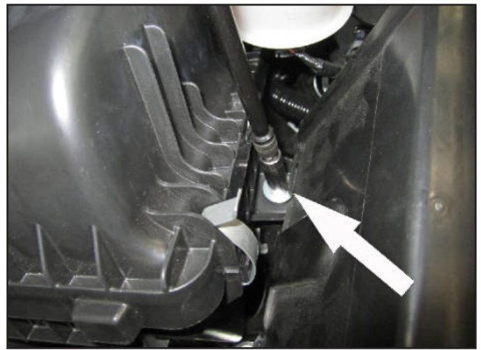
b. Remove the right 10mm bolt securing the factory air box.
