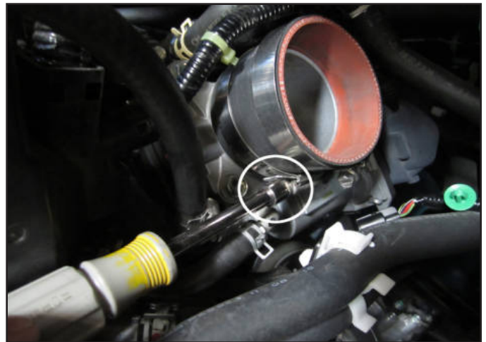
g. Tighten the hose clamp on the throttle body.
