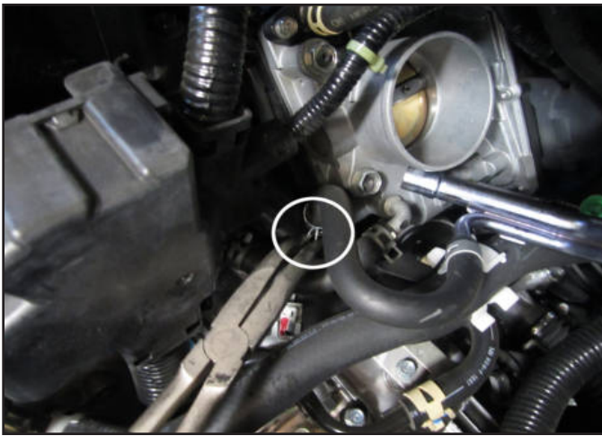
af. Release the clip on the throttle body hose and move upward.
