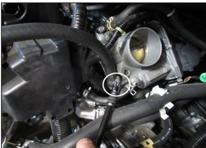
d. Tighten the 1/4" hose clamp on the throttle body inlet as shown.
