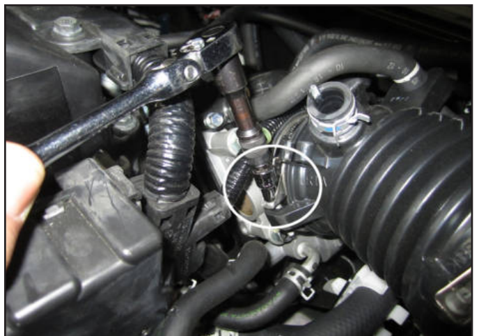
t. Loosen the hose clamp at the throttle body.
