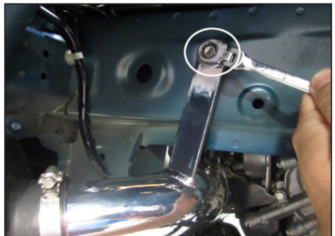
q. Tighten the 10mm nut on the lower intake tube mount. (Ensure there is no contact with any engine or body component).
