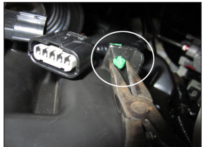
h. Release the mass air sensor clip on the air box.
