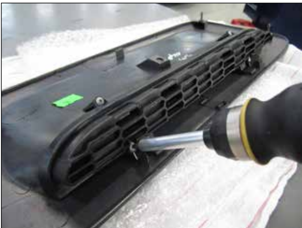
e. Place the bezel face down on a soft cloth or towel and remove the 4 small Phillips screws retaining the air restrictor grille. Remove the grille.
