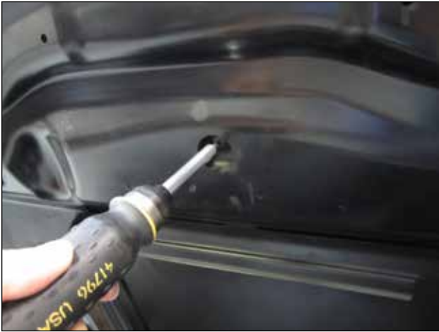
a. Open the vehicle hood (bonnet). Loosen the screw clip under the front of the hood.
