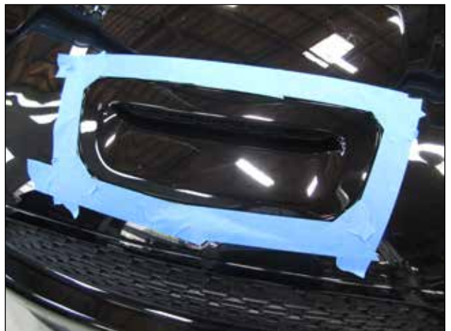
f. Re-install the now fully open bezel by hand. Open the hood and re-install the screw clip.
