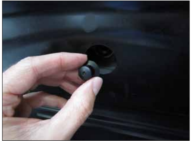
b. Carefully remove the screw clip retaining the stock hood inlet bezel and close the vehicle hood.
