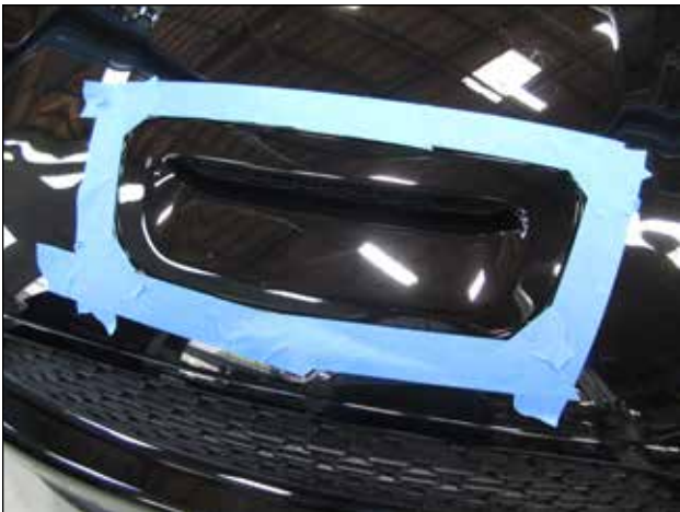
c. Applying tape around the bezel before removal to protect the hood's finish is recommended.
