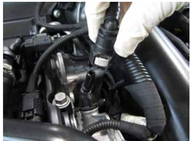
d. Disconnect the vacuum line port.
