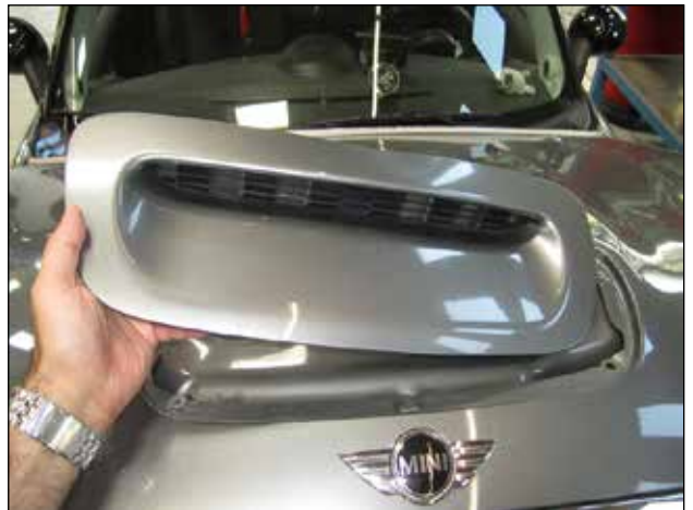
d. Carefully pull up at the rear center of the inlet bezel using small finger tips and a soft cloth to protect the finish. Then pull up on the remaining mounting tabs to remove the bezel assembly.
