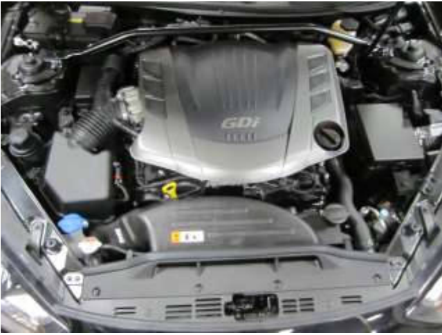
STOCK INTAKE INSTALLED
