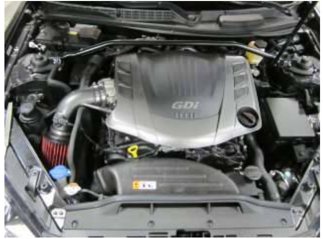
AEM INTAKE INSTALLED
