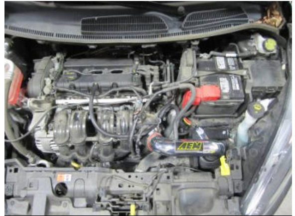
AEM Intake Installed
