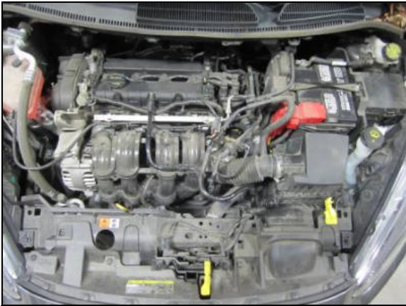
Stock Intake Installed
