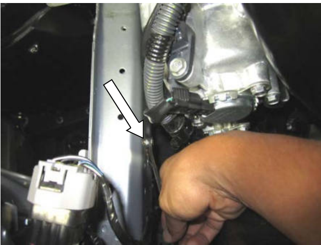
i. Remove the M6 ground bolt located on the lower frame rail and set aside for use with AEM heat shield.
