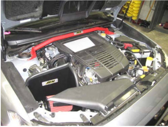
n. AEM intake installed.
