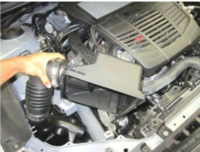
g. Slide the intake tube off the lower bellow coupler and remove tube/box assembly from engine bay.
